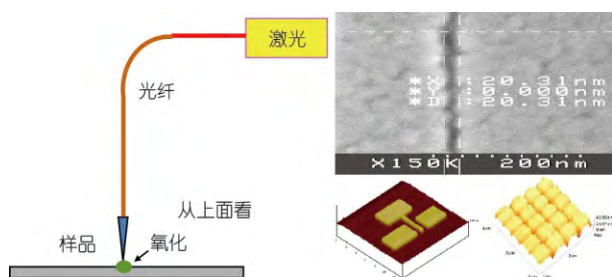
图8 (网络版彩图)激光和近场显微镜组合 Figure 8 (Color online) Combination of laser and near-field microscope for nanolithography.
