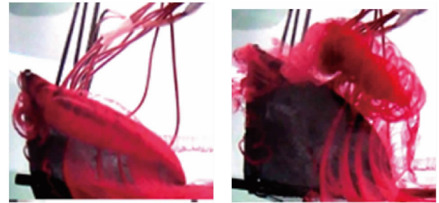
图 6 U_\infty = 10 \text{ mm/s} 时的脱落涡 Fig. 6 Shedding vortex system at U_\infty = 10 \text{ mm/s}
