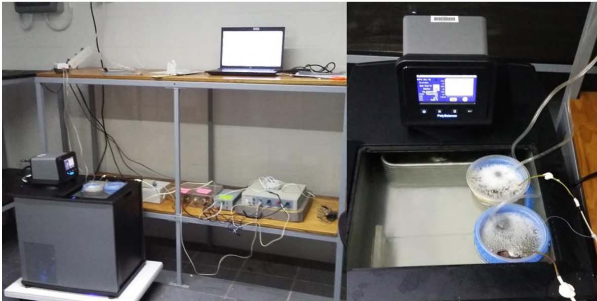
Figure 5.2. Experimental setup for measuring heart rate activity with an increase in temperature for mussels Perna perna and crabs Parasesarma catenatum (left) whereby infrared sensors were attached to mussels/crabs and placed in 100 ml aerated containers floated in a programmable water bath (right).
