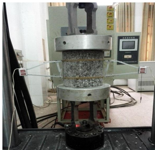
Figure 6. Device of compression resilience modulus test.
