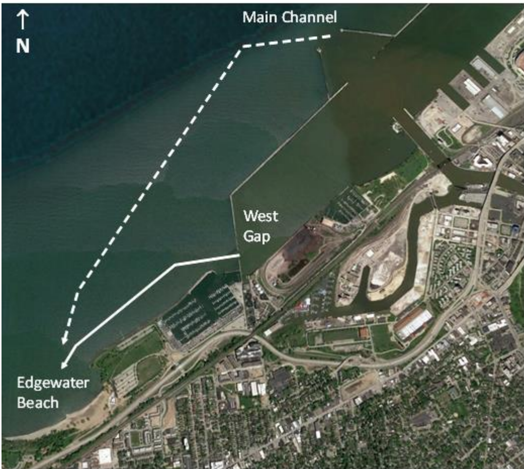
Figure 12 - Position of breakwall at the mouth of the Cuyahoga River and potential paths of plumes reaching Edgewater Beach.
