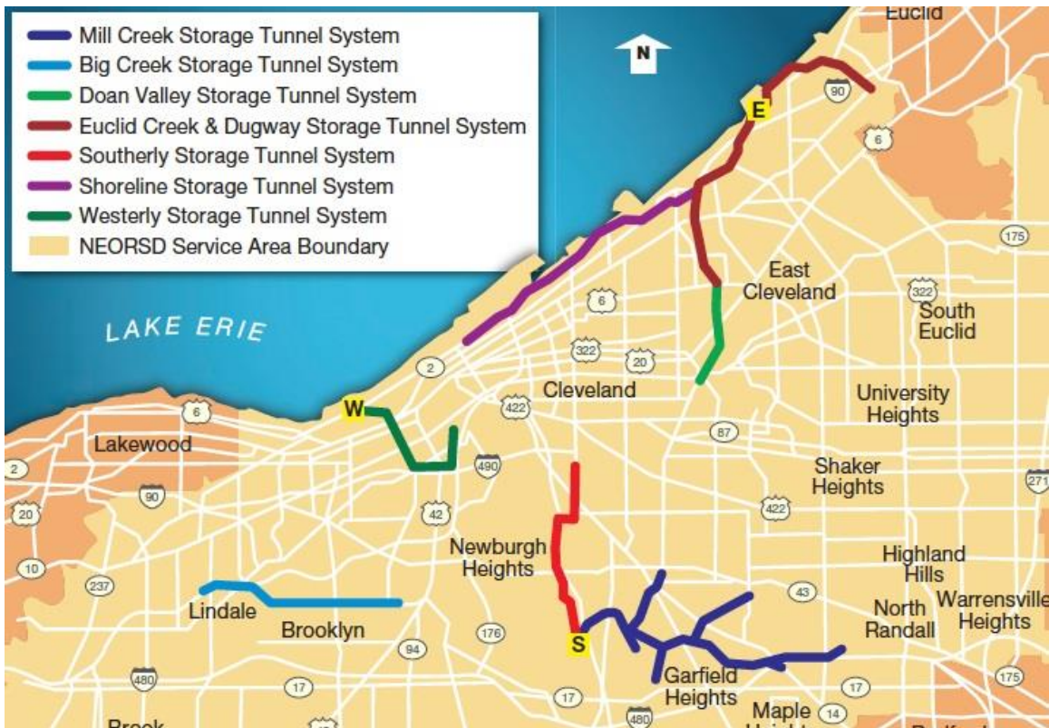
Figure 1 - The Northeast Ohio Regional Sewage District service area, including the location of tunnel systems and wastewater treatment plants (W, Westerly, S, Southerly and E, Easterly).
