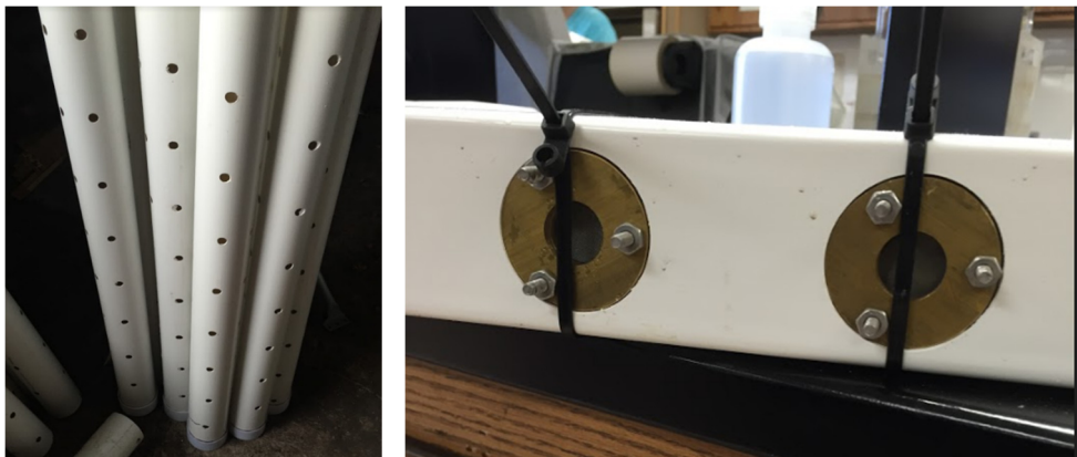
Figure 2-11. Installation of poliovirus sentinel chambers in pilot-scale boxes. A) Pipe in pipe design and B) poliovirus sentinel chamber installation.
