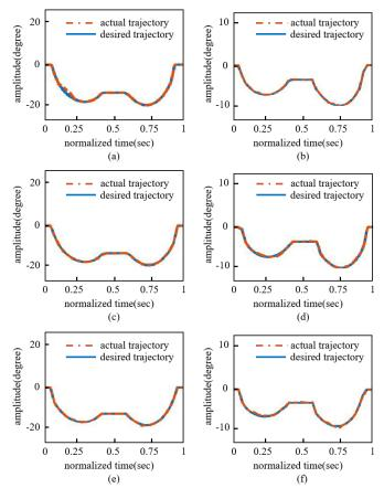
Fig. 14. Experimental results of three subjects.(a), (c), and (e) are the knee's tracking trajectories of subjects 1, 2, and 3, respectively. (b), (d), and (f) are the ankle's tracking trajectories of subjects 1, 2, and 3, respectively
