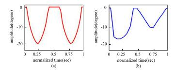
Fig. 7. The change of knee joint in Case S1.(a)the fixed motion of leg prosthesis.(b)the real motion of contralateral leg at the same time.
