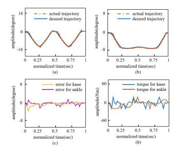
Fig. 11. Experimental results of subject 3.(a)The tracking trajectory of knee joint.(b)The tracking trajectory of ankle joint.(c)The trajectory error.(d)The torque of each joint
