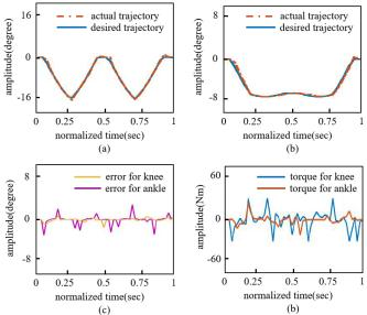
Fig. 9. Experimental results of subject 1.(a)The tracking trajectory of knee joint.(b)The tracking trajectory of ankle joint.(c)The trajectory error.(d)The torque of each joint
