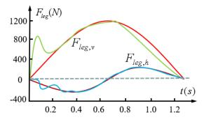
Fig. 1. Ground reactive force (GRF) of the contralateral leg during stance phase
