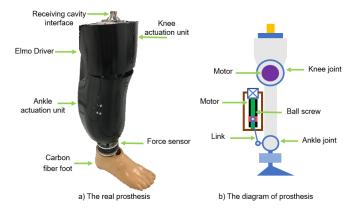
Fig. 6. The mechanical structure of the leg prosthesis
