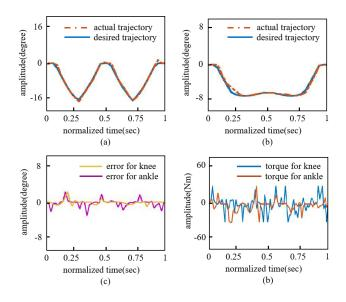
Fig. 10. Experimental results of subject 2.(a)The tracking trajectory of knee joint.(b)The tracking trajectory of ankle joint.(c)The trajectory error.(d)The torque of each joint
