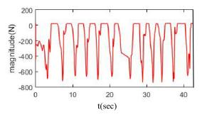
Fig. 12. Ground reactive force under level ground
