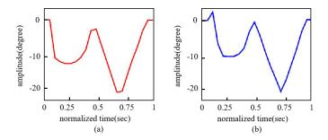
Fig. 8. The change of knee joint in Case S2.(a)the real trajectory of the leg prosthesis' knee joint which imitates the motion of contralateral leg.(b)the desired trajectory of the leg prosthesis' knee joint generated from the proposed method.
