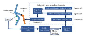
Fig. 3. The diagram of the proposed control method
