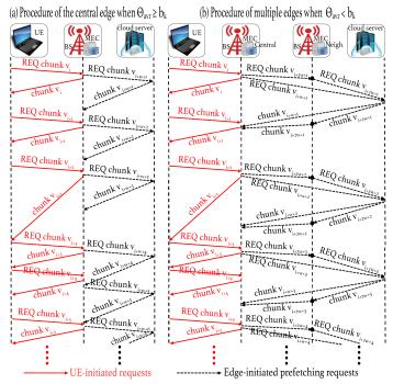
Fig. 2: Illustration of the proposed pre-fetching scheme
