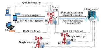
Fig. 1: Proposed System Architecture
