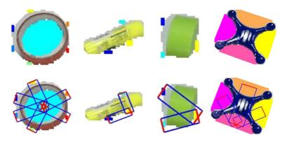
**Fig. 5** Results for morphological image processing. The colorful area is marked as the regions of interest. And the bottom part samples some candidate rectangles for four types of objects
