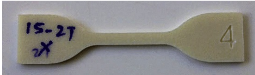
Fig. 4 A fabricated tensile specimen.
