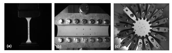
Fig. 2. Multi deformation-mode mechanical characterisation in (a) uniaxial, (b) planar and (c) equibiaxial tension.
