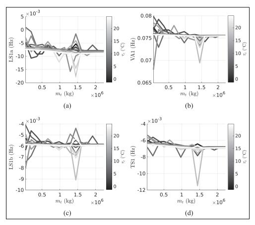
Figure 9. Prediction of the Tamar bridge natural frequency (a) LSIa, (b) VAI, (c) LSIb and (d) TSI discrepancy function for varying temperature (grayscale lines) and traffic (abscissa) conditions.
