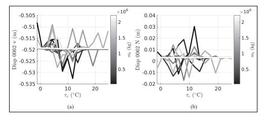
Figure 10. Prediction of the Tamar bridge mid-span (a) vertical and (b) Northern displacement discrepancy function for varying temperature (abscissa) and traffic (grayscale lines) conditions.
