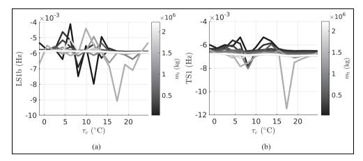
Figure 11. Prediction of the Tamar bridge natural frequency (a) LS1b and (b) TS1 discrepancy function for varying temperature (abscissa) and traffic (grayscale lines) conditions.
