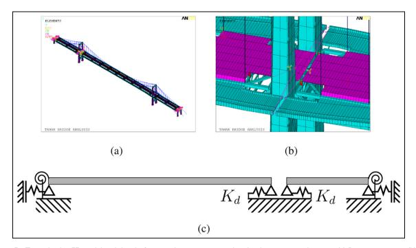
Figure 5. Tamar bridge FE model and detail of imposed constraints simulated as linear spring elements. (a) Perspective view, (b) expansion gap at Saltash tower and (c) bridge boundary conditions diagram.
