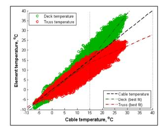
**Figure 6.** Assumed temperature relations between cable, shaded and lighted groups for Tamar bridge FE model and associated monitored data.
