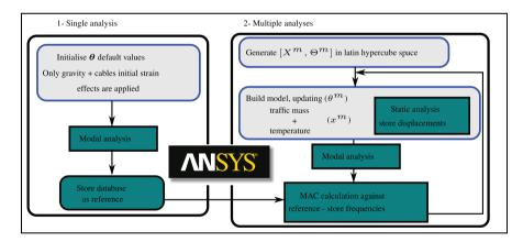
Figure 7. Simulation flowchart.
