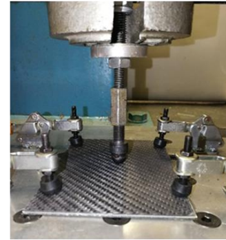
Figure 2. a) Diagram of a low-velocity test rig, b) Low-velocity test rig (impact tower), d) Clamped sample and impactor, and c) ASTM standard clamp and test set up.
