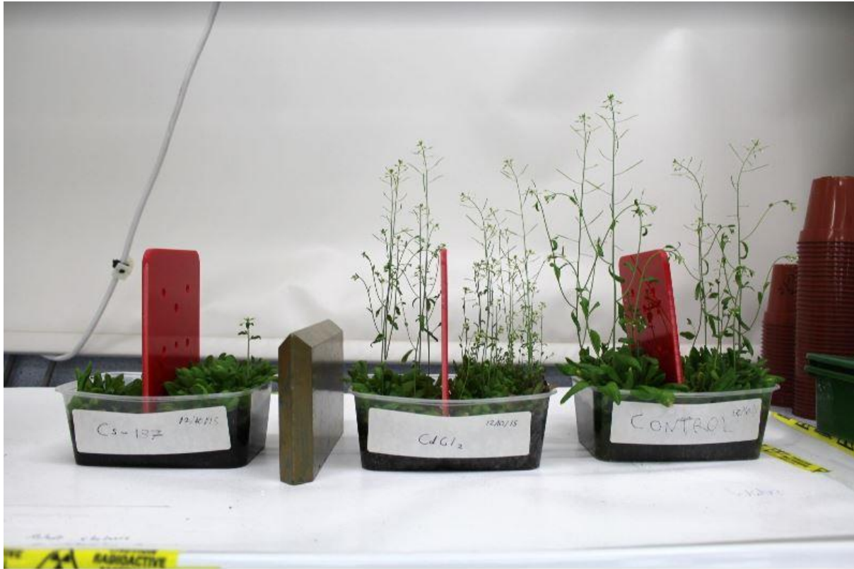
Fig. 2.5. Preliminary experiment (generation 4) with Cs-137 treatment (left), CdCl 2 (centre) and negative control (right) in a trial configuration in small plastic containers with sparsely sown and densely sown plants in the same container, separated with a plastic divider. High-density lead blocks (located between the Cs-137 container and the CdCl 2 container) were used at all times to shield control group plants from ionising radiation.
