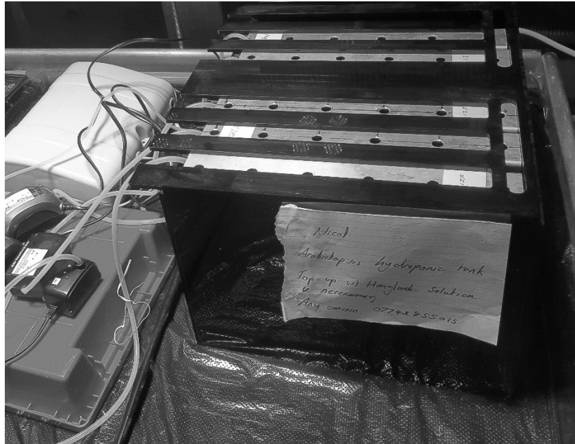
Fig. 2.15. Hydroponic tank with aeration system setup. Spaces for six inserts (housing 5 samples) built into the design with a large diameter space between three inserts capable of housing a lead sheet for sample shielding against gamma rays.
