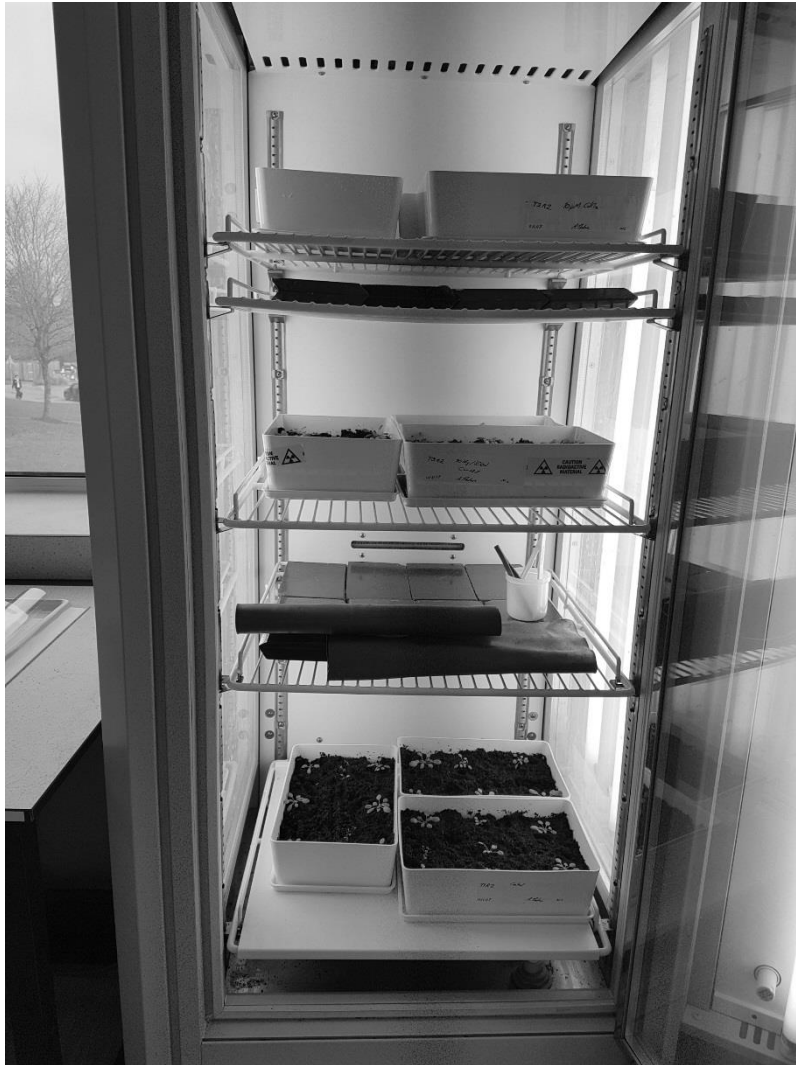
Fig. 2.7. Final layout of containers in growth cabinet (Panasonic MLR-352/352H) set at a day length of 16 hours of light at 22 °C/14°C and 70% humidity. Note the bulge in the second shelf from the top that held the lead shielding. This is due to the weight of the shielding. A plastic beaker containing plastic tweezers is also pictured on the fourth shelf from the top (which also had a layer of lead shielding) and this was for removal of any unwanted plants (i.e. germinated plants hidden beneath the leaves of the deliberately placed replicates).
