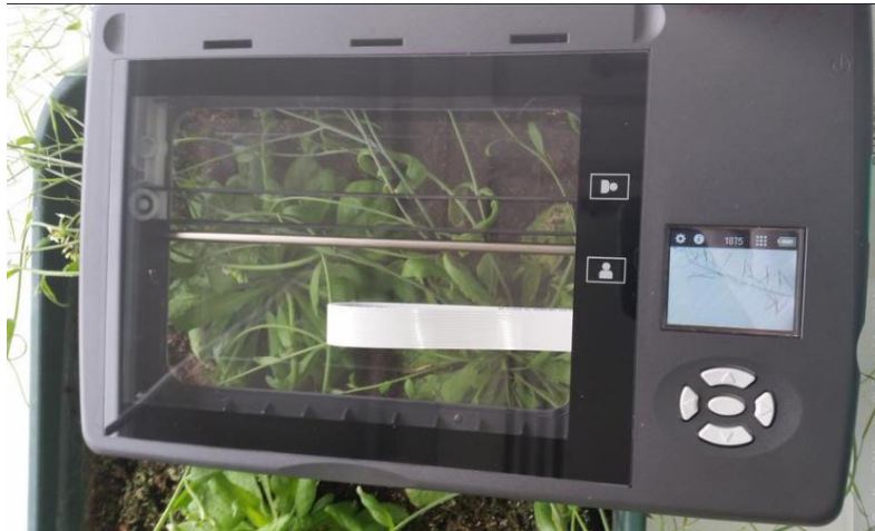
Fig 3.2. Doxie Flip scanner shown during a scan with the lid removed. The live view screen displays scans in real time for accuracy purposes. The control panel allows the user to review images prior to storage and upload.
