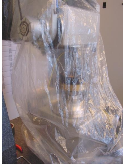
Figure 51: Foil covered SCMM. In a first attempt, the SCMM was covered with a simple foil. This primitive cover had the goal to minimise the volume around the measurement area of the SCMM and to protect against turbulence. Furthermore, the parameters of the climate control had been changed from \pm 1K temperature tolerance to \pm 0.25K and the hysteresis of the climate control system from 600 seconds to 300 seconds
