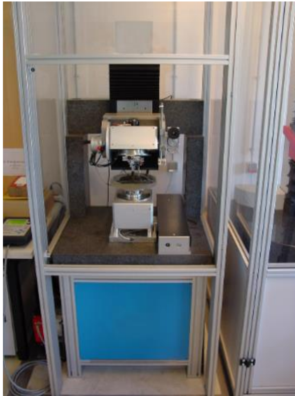
Figure 53: Housing of the SCMM. The stable housing with Plexiglas™ replaces the first simple foil cover.
