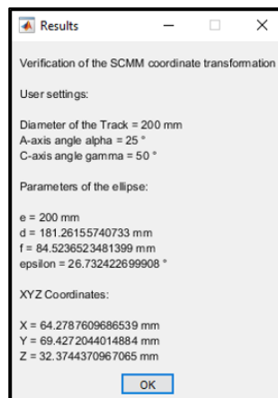
Figure 27: XYZ verification with Matlab™ (M2010a). Comparable to the verification of the A-axis angle \alpha , the verification of Equation 11 to Equation 16 was performed with Matlab™ (M2010a) and Creo™. Both software tools calculated with the same presented input parameters.
