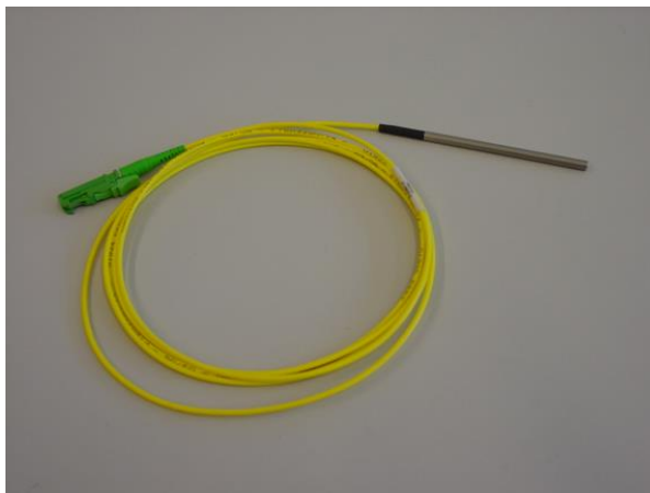
Figure 87: MicroEpsilon™ Confocal chromatic sensor [79]
