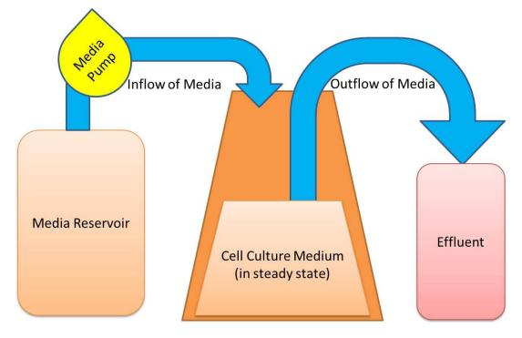
Figure 5.1 - Graphical representation of the chemostat method/biofilm continuous culture reactor for culturing bacterial cells.
