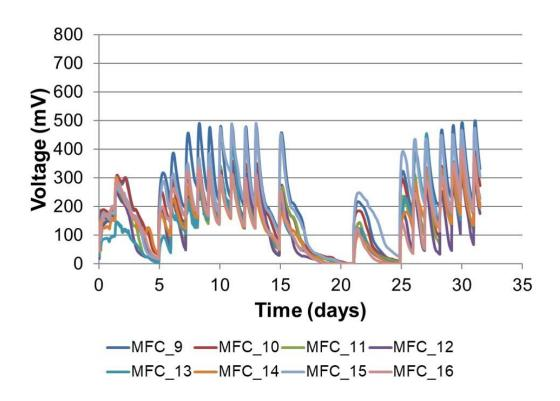
Figure 5.25 – Long-term temporal voltage behaviour of the manually maintained MFCs.
