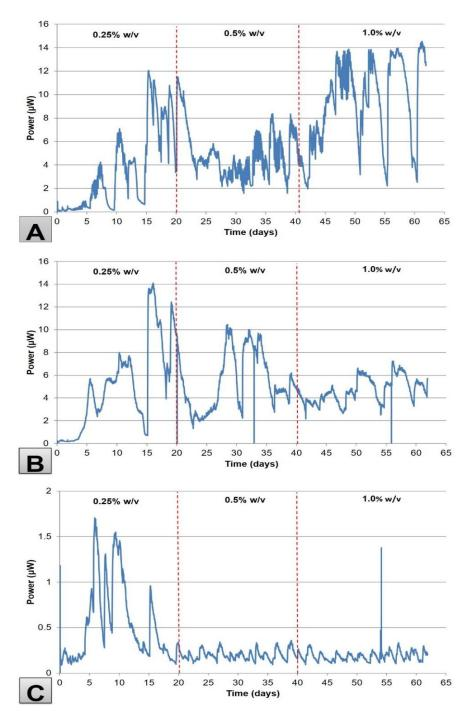
Figure 5.9 – Temporal power output of [A] acetate, [B] lactate and [C] cellulose fed MFCs, at different concentrations, via the EvoBot.
