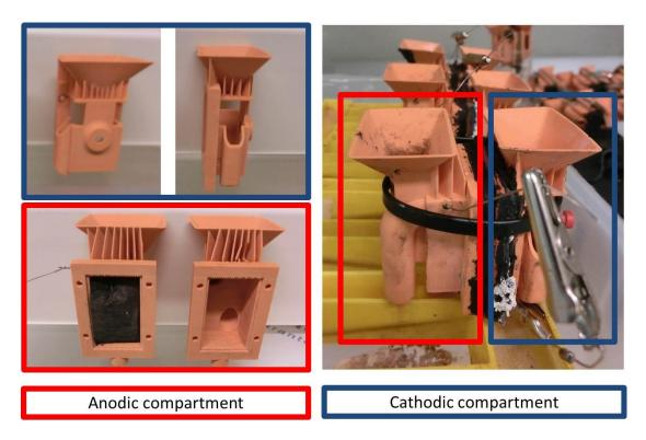
Figure 3.4 - 3D printed small-scale MFCs.
