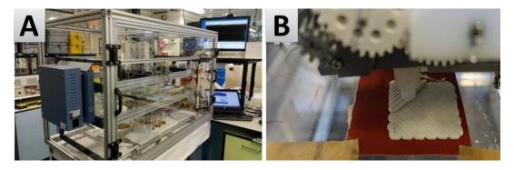
Figure 4.11 - EvoBot RepRap 3D-printer.
