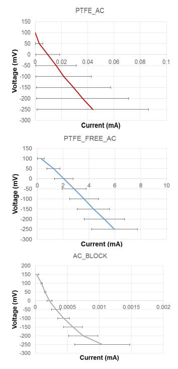
Figure 4.26 – Linear sweep voltammetry results of the three cathode electrodes (250 mV/S) (n=3).
