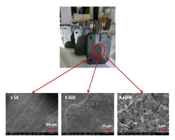
Figure 4.4 - SEM images at three different magnification of the MEA side surface coated with the graphite ink (cathode side).
