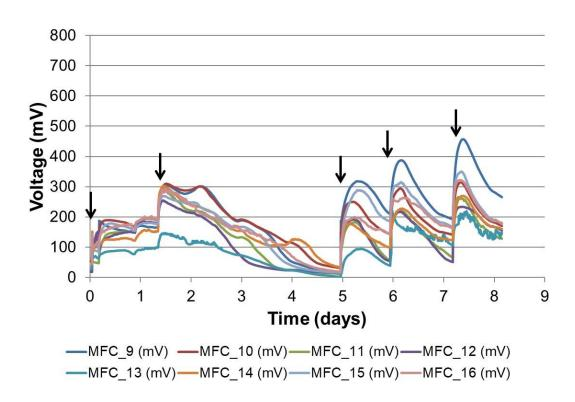
Figure 5.23 - Temporal voltage behaviour of the MFCs maintained manually and fed once a day (batch-mode feeding).
