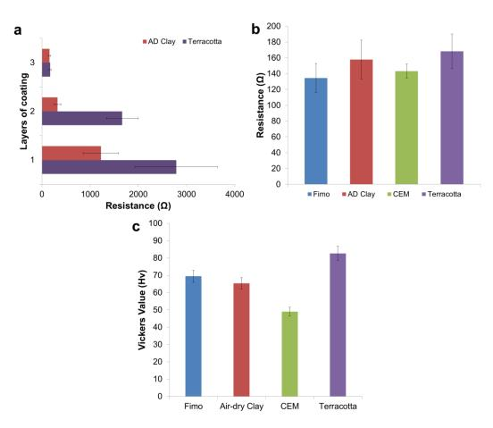
Figure 4.5 - Resistivity of the MEA and hardness of the membrane.
