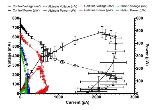
Figure 4.19 - Power curves produced after two months operation on a fixed load of 2.7  $k\Omega$
