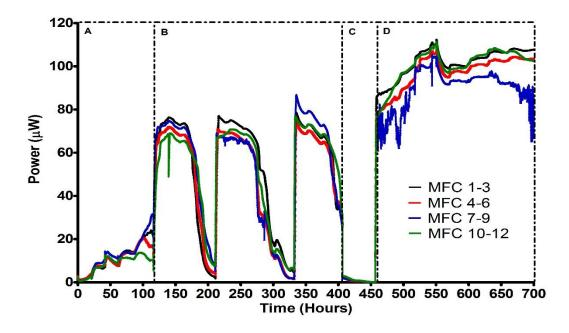
Figure 4.15 - Power profile of the inoculation process and initial feeding of the twelve MFCs.
