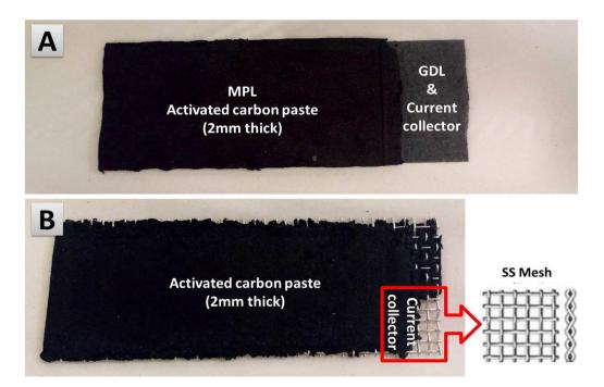
Figure 3.1 - Photos of the two mainly used types of air-breathing cathode electrodes in this study.
