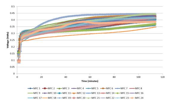
Figure 5.13 – OCV of 24 individually fed MFCs inoculated by EvoBot with activated sludge.
