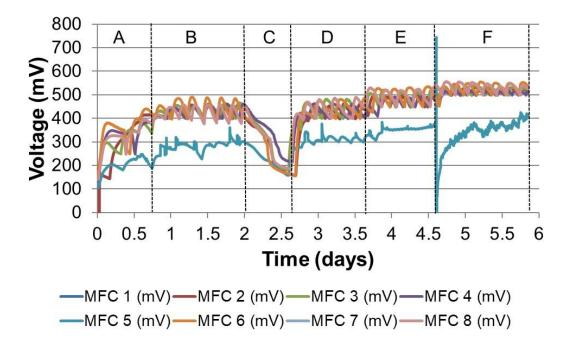
Figure 5.24 – Temporal voltage behaviour of the MFCs maintained by the EvoBot robot and based on different threshold values under 2.7 k $\Omega$  load.
