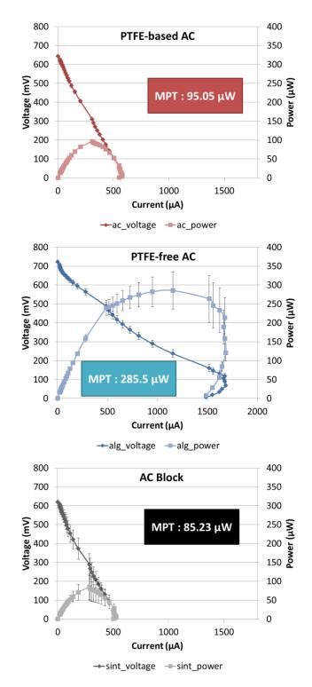
Figure 4.25 – Polarisation results of the three types of MFCs examined. (n=3)
