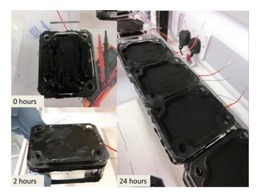
Figure 4.22 - Manually extruded PTFE-free alginate electrode 0, 2 and 24 hours after extrusion, showing the electrode settling and solidifying (air-drying).
