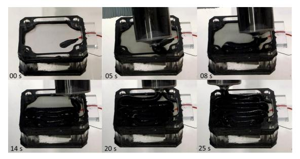
Figure 4.21 – Time-lapse photography of the manual extrusion of the PTFE-free/alginate based cathode electrode on the membrane of an assembled MFC.
