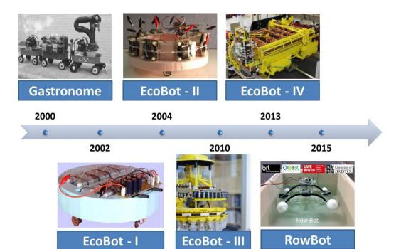
Figure 2.10 – MFC powered autonomous robots in chronological order until 2015.
