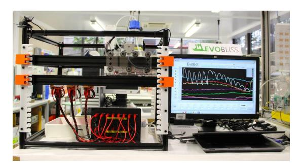
Figure 2.11 – EvoBot robotic workstation
