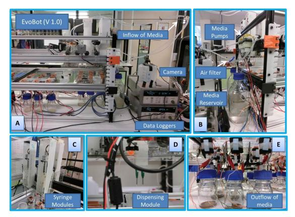
Figure 5.11 – Improved EvoBot based on the Chemostat approach for Phase III experiments.
