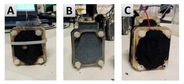
Figure 4.20 – Photographs of the three different cathode electrodes used in this study.
