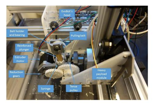
Figure 4.12 - Universal paste extruder mounted on a heavy payload module on the EvoBot robotic head.
