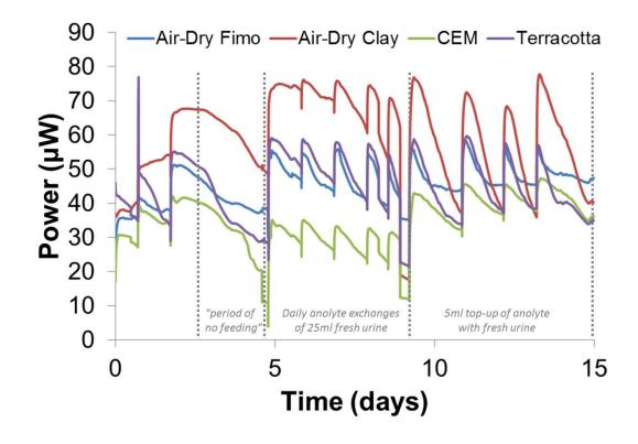
Figure 4.6 - Power generation recorded in the first 15 days of operations.
