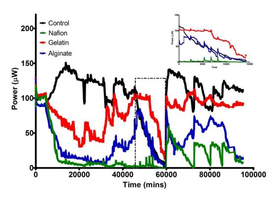
Figure 4.17 - Average power production of MFCs after feeding with different soft materials.
