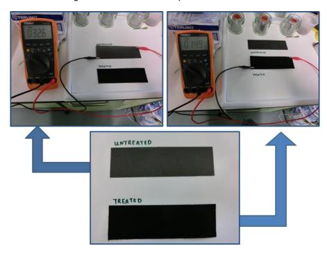
Figure 5.21 – Treated and untreated carbon veil electrode and their resistance.
