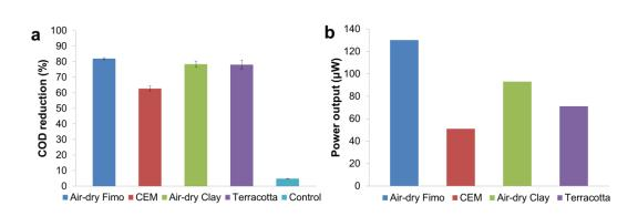
Figure 4.9 - COD reduction results and power output at the time of sampling.
