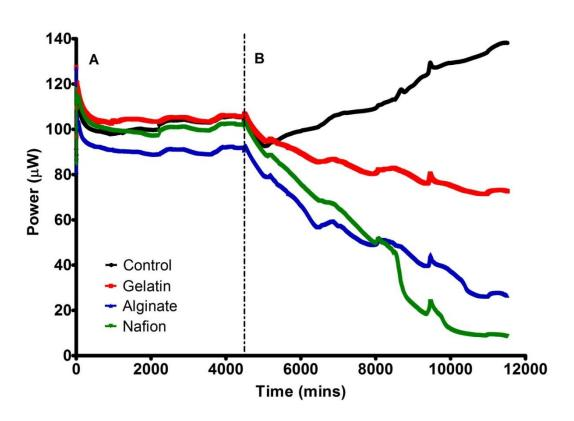
Figure 4.16 - Time profile of MFC's after feeding with soft materials for the first time.
