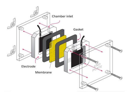
Figure 2.3 - Re-drawn version of the Microbial Fuel Cell prototype as created by Allen and Bennetto in 1993.
