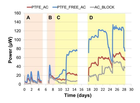
Figure 4.23 – Temporal power output of the MFCs employing different cathode electrodes.
