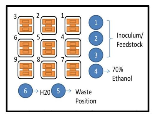
Figure 5.5 – Layout of Phase II experiment on EvoBot platform.
