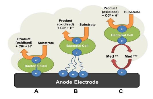
Figure 2.6 - Schematic representation of direct (A & B) and indirect (C) electron transfer between bacterial cells and anode electrodes.
