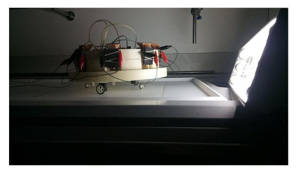
Figure A.3 Photo of EcoBot-II 2018 edition (from the side) performing phototaxis.
