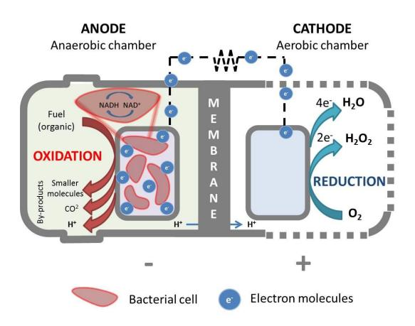
Figure 2.4 - Schematic representation of a Microbial Fuel Cell showing the reduction and oxidation (Redox) processes in each compartment.
