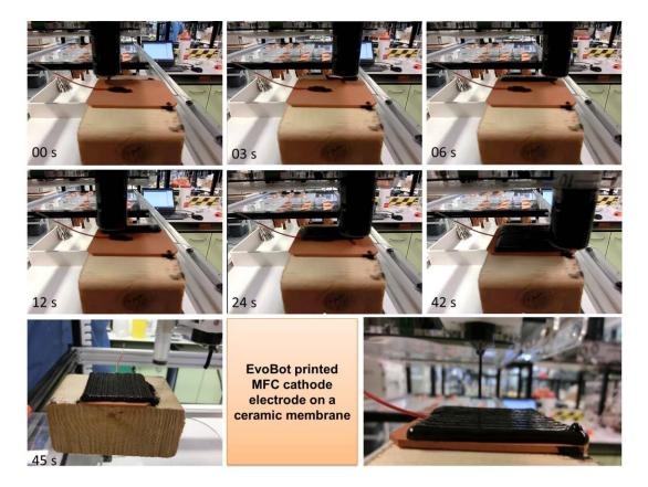
Figure 4.27 - Time-lapse photographs of the EvoBot extrusion of the PTFEfree/alginate based cathode electrode on a ceramic MFC membrane.
