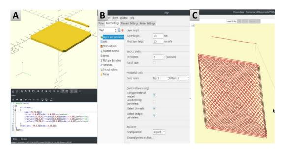
Figure 4.13 - The process of 3D printing membranes.
