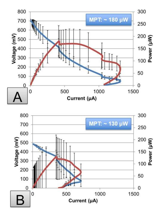
Figure 5.26 – Mean (n=8) polarisation results gathered on the 6th day of operation. [A] EvoBot matured MFCs [B] Manually/ Bench matured MFCs
