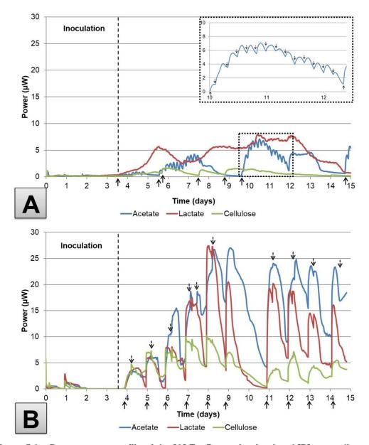
Figure 5.8 – Power output profile of the [A] EvoBot maintained and [B] manually maintained MFCs for a time period of two weeks.
