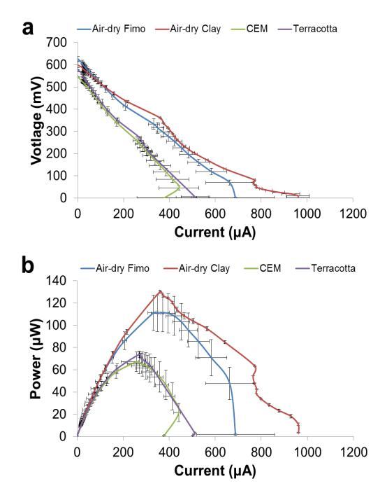
Figure 4.8 - Polarisation results [A] voltage vs current curve and [B] power curve. (n=3)
