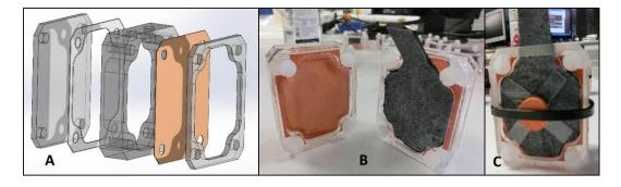
Figure 4.14 - MFC design and set-up.
