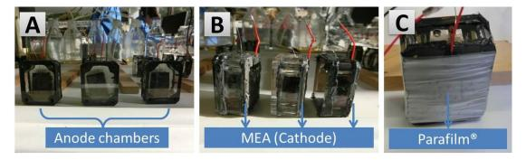
Figure 4.2 - Photographs of the MFC setup.
