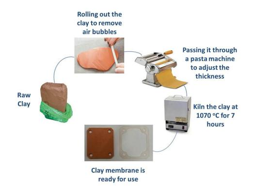
Figure 3.2 - In-house preparation technique for custom made clay membrane "kilned clay".
