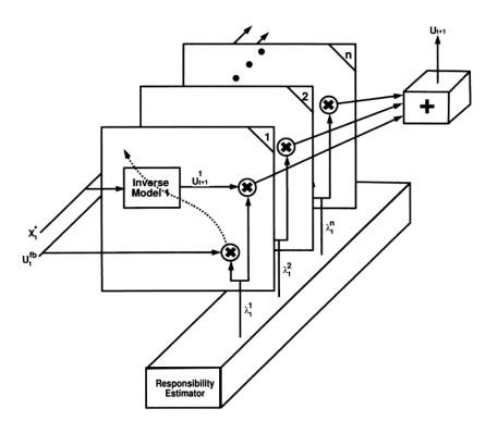
Figure 27. Multiple models showing only inverse models. Reprinted from [6]  $\bigcirc$  1998, with permission from Elsevier.
