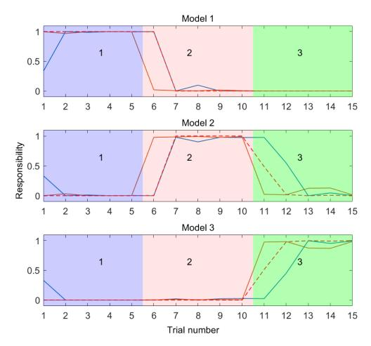
Figure 45. RP output with 6 audio features manually selected. The orange curve is RP output, the blue curve is posterior responsibility, the red broken curve is the combined responsibility.
