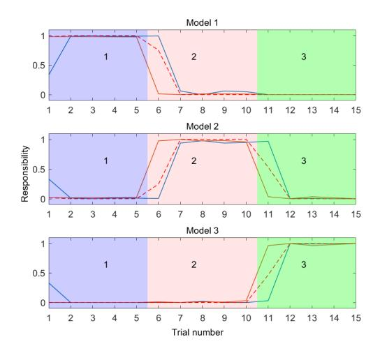
Figure 44. RP output with 1 audio feature (mean zero crossing rate). The orange curve is RP output, the blue curve is posterior responsibility, the red broken curve is the combined responsibility.
