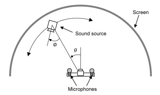
Figure 31. Plan view of the experimental apparatus. The source can be placed at various azimuths  $\theta$  with respect to the robot head. The sound source can also be rotated at an angle  $\phi$  on its axis. Reprinted from [54]. © 2018 IEEE.
