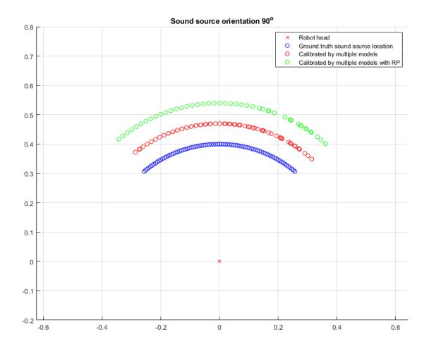
Figure 73. Results of cerebellar calibration post-learning: multiple models with RP (green circles) versus multiple models without RP (red circles). Blue circles are ground truth sound source position. Axes show x,y distance in metres with robot head at the origin. Context is  $\phi = 90^{\circ}$ .
