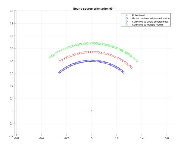
Figure 70. Results of cerebellar calibration post-learning: multiple models (green circles) versus a single general model which has learned in all contexts (red circles). Blue circles are ground truth sound source position. Axes show x,y distance in metres with robot head at the origin. Contexts is  $\phi = 90^{\circ}$ .
