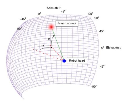
Figure 4. Audio map of sound source location in head-centric space. Reprinted from [54]. © 2018 IEEE.
