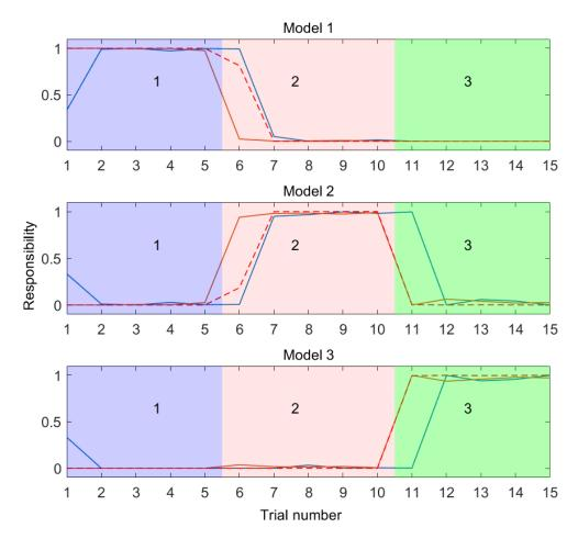
Figure 46. RP output with features selected using sequential feature selection. The orange curve is RP output, the blue curve is posterior responsibility, the red broken curve is the combined responsibility.
