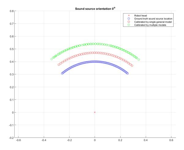
Figure 69. Results of cerebellar calibration post-learning: multiple models (green circles) versus a single general model which has learned in all contexts (red circles). Blue circles are ground truth sound source position. Axes show x,y distance in metres with robot head at the origin. Contexts is  $\phi=0^{\circ}$ .
