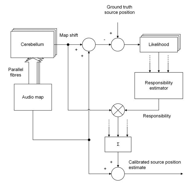
Figure 33. Multiple-models- inspired audio localisation. For a given context, each model provides an estimate of source position. The RE produces a responsibility signal for each model, based on the posterior likelihood calculation. The overall map shift is produced from a summation of model map shifts in proportion to their responsibility. Reprinted from [54]. © 2018 IEEE.
