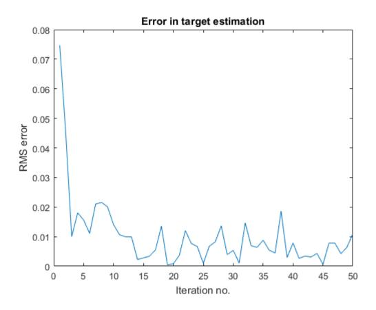
Figure 20. Error in target estimation during learning. y axis units are metres: distance along azimuthal arc from  $0^{\circ}$ .
