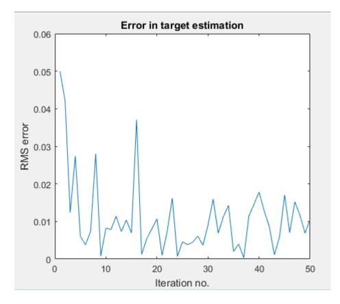
Figure 23. Error in target estimation during learning, using vision. y axis units are metres: distance along azimuthal arc from  $0^{\circ}$ .
