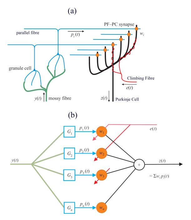
*Figure 8. Adaptive filter model of the cerebellum. (a) Cerebellar microcircuit. (b) Adaptive filter equivalent. Adapted with permission by Royal Society from [7].*
