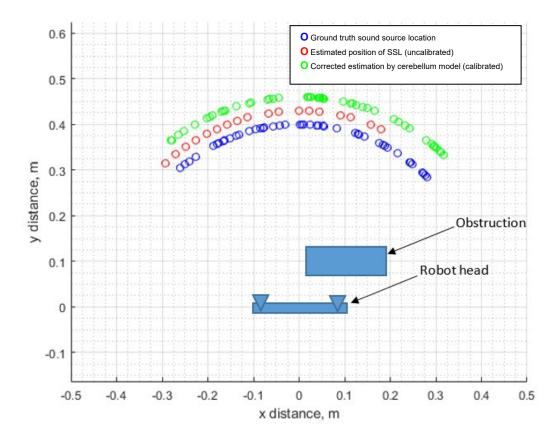
Figure 19. Results of cerebellar calibration in learning mode. One microphone is obscured. Estimated position (red) and calibrated (green) are offset in the y direction for clarity. Calibrated positions show learning (update of cerebellar parallel fibre/Purkinje cell weights) over 50 iterations.
