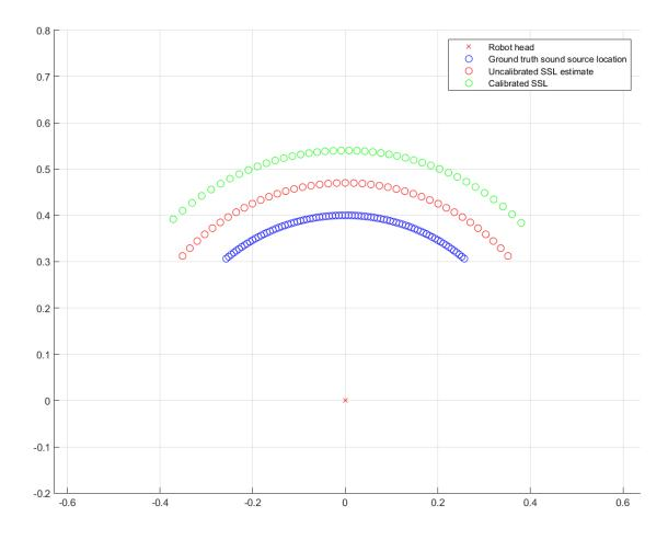
Figure 67. Results of cerebellar calibration post-learning: cerebellar calibration (green circles) versus uncalibrated SSL estimate (red circles). Blue circles are ground truth sound source position. Axes show x,y distance in metres with robot head at the origin.
