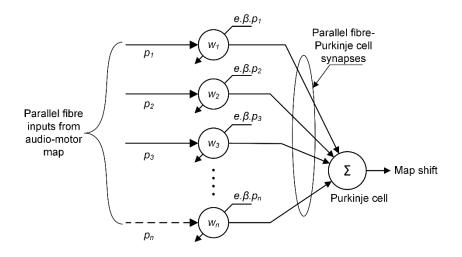
*Figure 12. Cerebellar calibration using the adaptive filter model of the cerebellum. Reprinted from [54].* © 2018 IEEE.
