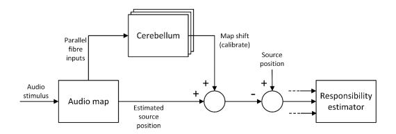
Figure 29. Multiple-models- inspired context estimation. For a given context, each model provides an estimate of source position. Each estimate is then compared to the ground truth source position and the RE classifies the acoustic context based on the estimation errors. Reprinted by permission from Springer Nature [113] © 2017.
