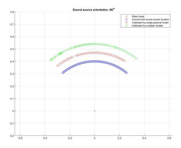
Figure 68. Results of cerebellar calibration post-learning: multiple models (green circles) versus a single general model which has learned in all contexts (red circles). Blue circles are ground truth sound source position. Axes show x, y distance in metres with robot head at the origin. Context is  $\phi = -90^{\circ}$ .
