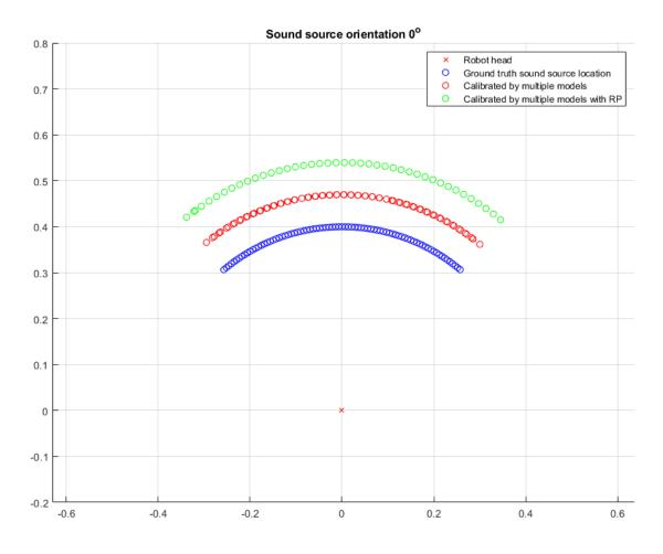
Figure 72. Results of cerebellar calibration post-learning: multiple models with RP (green circles) versus multiple models without RP (red circles). Blue circles are ground truth sound source position. Axes show x,y distance in metres with robot head at the origin. Context is  $\phi = 0^{\circ}$ .
