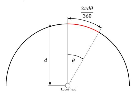
Figure 13. Internal representation of azimuth.
