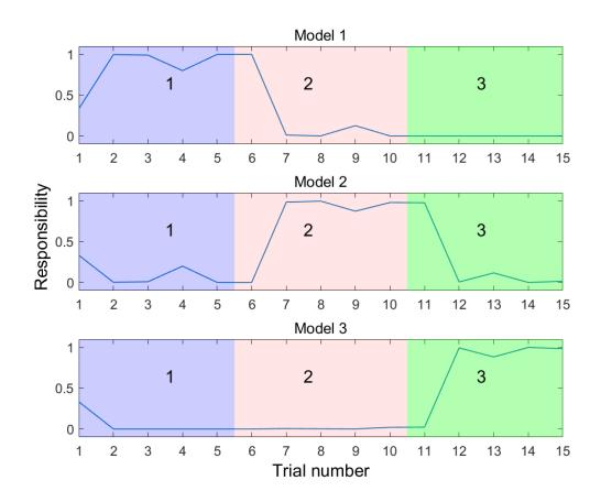
Figure 36. Responsibility signals as the system progresses through the 15 trials. In each trial the system is presented with stimulus of various azimuths in three different contexts, indicated by the coloured regions, labelled with the context number. Context 1 (blue region) is  $\phi$ =900 left; context 2 (red region) is  $\phi$ =0°; context 3 (green region) is  $\phi$ =90° right. Reprinted from [54]. © 2018 IEEE.
