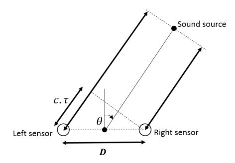
Figure 5. Determining azimuth  $\theta$  from Inter-aural Time Difference of arrival. c is the velocity of sound,  $\tau$  is the ITD and D is the inter-aural distance. A planar sound wave is assumed.
