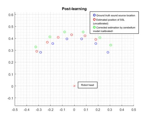
Figure 21. Results of cerebellar calibration post-learning. Axes show x,y distance in metres with robot head at the origin. Green points show calibrated estimates of source azimuth with learned weights applied to a new set of regularly spaced positions.
