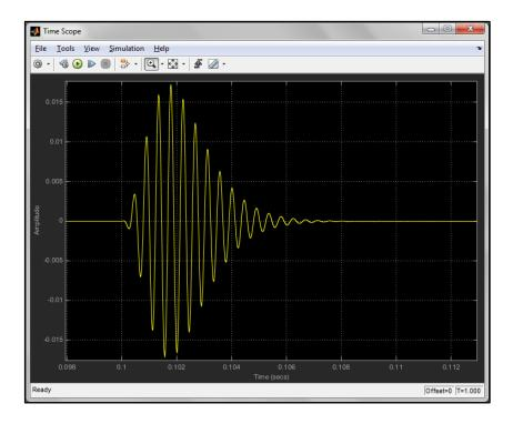
Figure 3. Impulse response of gammatone biquad filter in Simulink.
