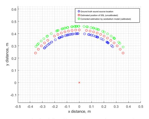
Figure 22. Results of cerebellar calibration in learning mode using vision. The SSL estimate is artificially distorted by multiplying SSL estimates by a factor of 1.3. Estimated position (red) and calibrated (green) are offset for clarity. Calibrated positions show learning (update of cerebellar parallel fibre/Purkinje cell weights) over 50 iterations.
