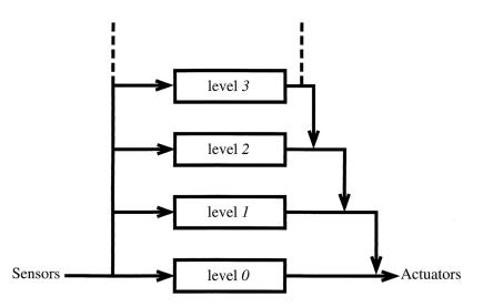
*Figure 7. Hierarchical layers in subsumption architecture. Reprinted with permission from [77].* © 1999 Massachusetts Institute of Technology, published by the MIT Press.
