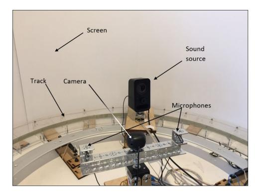
Figure 30. Experimental apparatus using track-mounted sound source. Adapted by permission from Springer Nature [113] © 2017.
