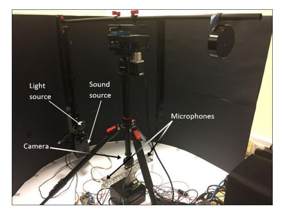
Figure 35. Experimental apparatus using tripod-mounted sound source. The sound source is suspended from a counterweighted beam, which rotates about the axis of the robot head. Reprinted from [54].  $\bigcirc$  2018 IEEE.
