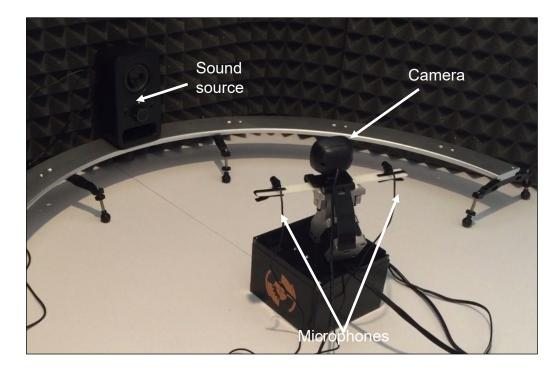
Figure 17. Experimental apparatus for the cerebellar calibration pilot experiments.
