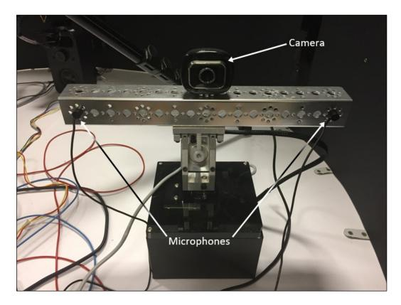
Figure 34. Robot head based on PTU. A horizontal bar with a microphone mounted at each extremity is mounted on a stepper motor to allow the head to orient toward the estimated azimuthal position of a sound source. Reprinted from [54]. © 2018 IEEE.
