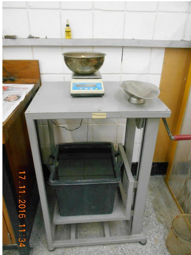
Figure 3-11 Laboratory set up of specific gravity and water absorption apparatus
