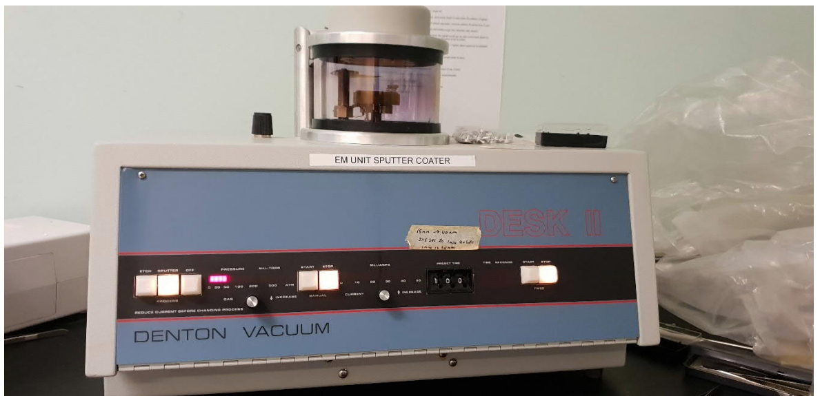
Figure 6-5 Denton Vacuum Desk II Sputter Coater [Reprint with permission from Monroe et al. (2019b)]
