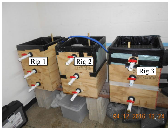
Figure 3-18 Three of four permeable pavement test rigs in the laboratory, December 2016 [Reprint with permission from Monrose et al. (2019a)]
