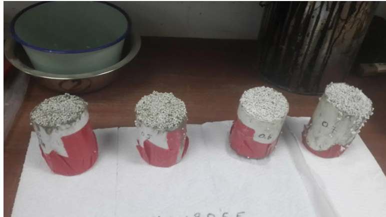
Figure 3-7 C-EPS samples for hydraulic conductivity testing, December 2016
