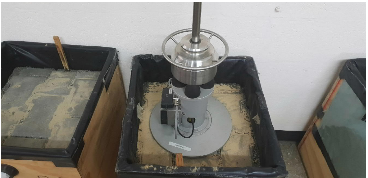
Figure 4-20 PFWD testing on one of the permeable pavement rigs in the laboratory
