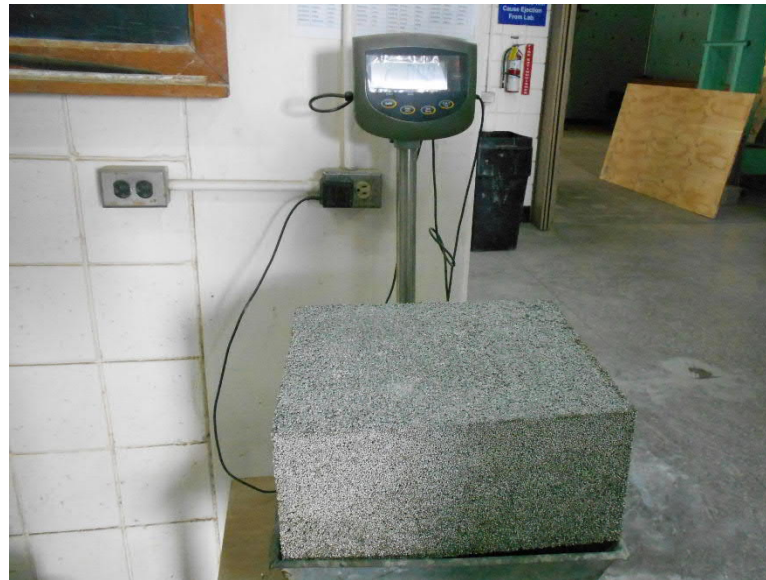
Figure 3-6 Block of C-EPS used as the sub-base layer in Rig 4, December 2016 [Reprint with permission from Monroe et al. (2019a)]
