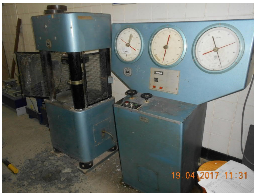
Figure 6-3 Concrete compressive and splitting tensile strength testing machine in laboratory
