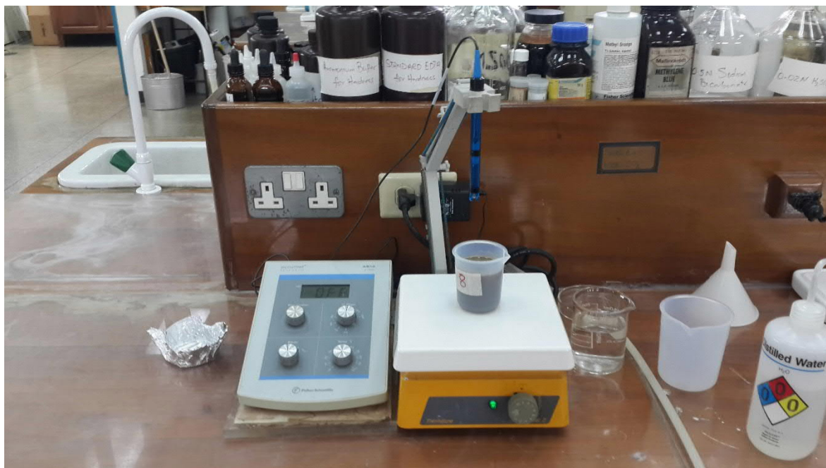
Figure 3-16 Fisher Scientific Accumet Research AR10 pH meter with sample in laboratory
