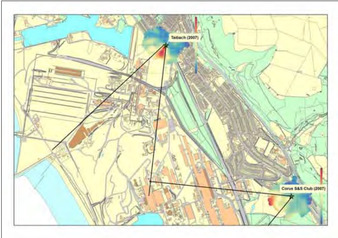
Figure 18: EAW Polar Plots Located on Local Area Map Indicating Likely Source Areas
