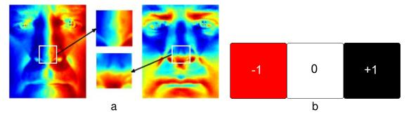
Figure 8.4: (a) illustrates the enlarged nose tip showing the x and y-components respectively, and (b) is the proposed basic filter for surface normals inspired by the Haar-like features used by Viola and Jones.
