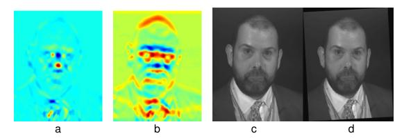
Figure 8.8: The nose tip region is highlighted (a) and used to mark the middle of the face along which the symmetry across the vertical axis of (b) is tested at different rotations. The rotation with the least amount of difference between the two sides is then applied to the original image (c) resulting in the roll corrected result shown in (d).
