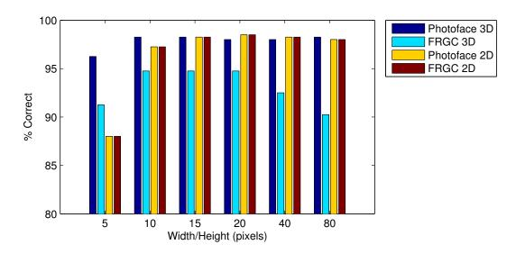
Figure 5.2: Performance of 2D (grey scale images from FRGC/albedo images from Photoface) and 3D (surface normal from both databases) face recognition on Photoface and FRGC data. No degradation in performance is produced even when resolutions are reduced to as little as  $10\times10$  px for 3D data and  $15\times15$  px for 2D data.
