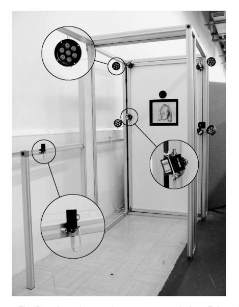
Figure 3.2: The Photoface photometric stereo capture device. Enlarged areas from top to bottom: NIR light source, a visible light source and an ultrasound trigger. The camera can be seen on the back panel above the monitor display.
