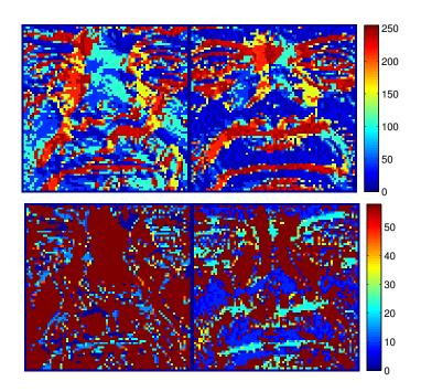
Figure 4.13: The top row shows an example of applying the LBP process to x and y components to give a 255 level LBP image. The bottom row shows the same results but with the commonly used 58 level image which employs the notion of uniform and non-uniform binary patterns.
