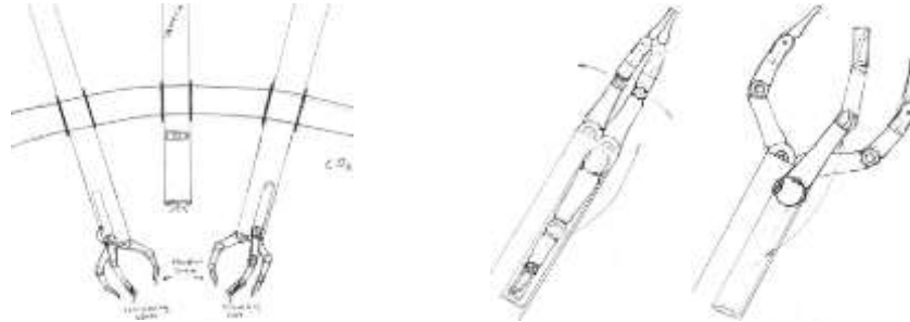
Fig. 1. a. Layout of instruments and camera inside the abdomen b. Folded – extended position
