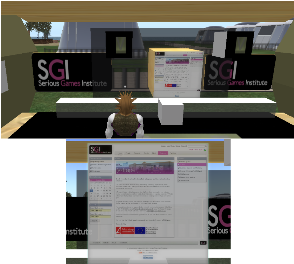
FIG. 1: An example of HTML on a prim in Second Life. Essentially creating an in-world web browser.
