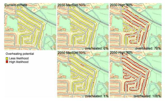
**Figure 7.12** Climate change impact as overheating potential for Bramhall at 2030s and 2050s climate periods, medium to high emissions, 50% to 90% probabilities (source: Digimap, 2012; The DECoRuM-Adapt model, 2012). Map@ Crown Copyright/database right 2012. An Ordnance Survey/EDINA supplied service.
