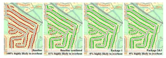
**Figure 7.14** Adaptation package results for 2050s, high emissions, 90% probability in Bramhall. Note: packages 2 and 3 do not differ in overheating reduction as package 3 is defined by the inclusion of solar energy systems alone (source: Digimap, 2012; The DECoRuM-Adapt model, 2012). Map@ Crown Copyright/database right 2012. An Ordnance Survey/EDINA supplied service.
