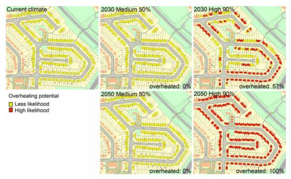
**Figure 7.13** Climate change impact as overheating potential for Cheadle at 2030s and 2050s climate periods, medium to high emissions, 50% to 90% probabilities (source: Digimap, 2012; The DECoRuM-Adapt model, 2012). Map@ Crown Copyright/database right 2012. An Ordnance Survey/EDINA supplied service.
