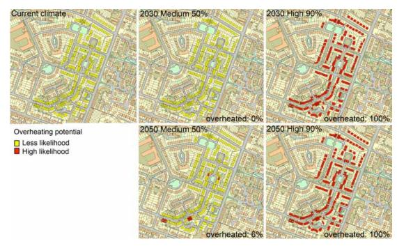
**Figure 7.4** Climate change impact as overheating potential for Upper Horfield at 2030s and 2050s climate periods, medium to high emissions, 50% to 90% probabilities (source: Digimap, 2012; The DECoRuM-Adapt model, 2012). Models reproduced under the terms of the Contractor's Licence for the Use of Ordnance Survey Data between UWE, Bristol and Bristol City Council. Map@ Crown Copyright/database right 2012. An Ordnance Survey/EDINA supplied service.
