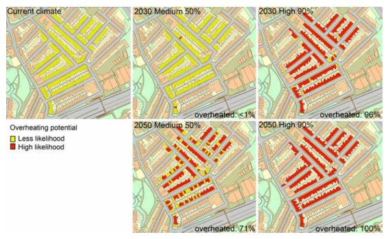
**Figure 7.3** Climate change impact as overheating potential for St. Werburghs at 2030s and 2050s climate periods, medium to high emissions, 50% to 90% probabilities (source: Digimap, 2012; The DECoRuM-Adapt model, 2012). Models reproduced under the terms of the Contractor's Licence for the Use of Ordnance Survey Data between UWE, Bristol and Bristol City Council. Map@ Crown Copyright/database right 2012. An Ordnance Survey/EDINA supplied service.
