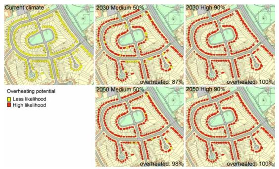
**Figure 7.7** Climate change impact as overheating potential for Botley at 2030s and 2050s climate periods, medium to high emissions, 50% to 90% probabilities (source: Digimap, 2012; The DECoRuM-Adapt model, 2012). Map@ Crown Copyright/database right 2012. An Ordnance Survey/EDINA supplied service.
