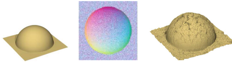
Fig. 1. A simple height map (left), its height gradient map with some noise added (middle) and the recovered height map (right) produced from the gradient by the Frail-Hancock tree-path integrator [32]. (In the gradient map, the X and Y derivatives are combined into color values.) (For interpretation of the references to color in this figure legend, the reader is referred to the web version of this article.)
