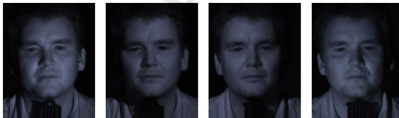
Fig. 4. Four images captured by PHOTOFACE after subtraction of ambient lighting and trimming by the face detection algorithm.
