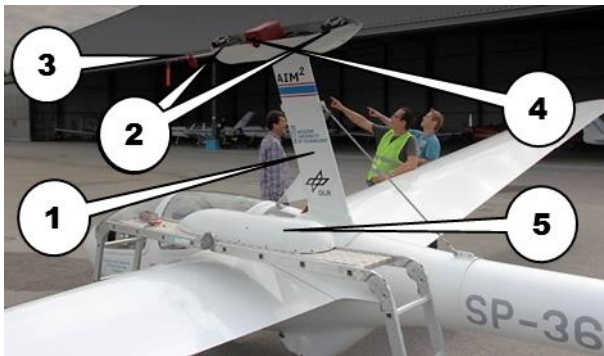
Figure 6 Dorsal camera pod installation on the PW-6U glider; (1) composite mast, (2) two IPCT cameras, (3) aerodynamic probe for pressure and \alpha - \beta -angle measurement, (4) one infrared thermography (IRT) camera, (5) disassembled housing cover
