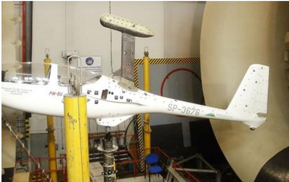
Figure 12 Glider fuselage with mounted camera pod, without wings and horizontal stabiliser in the working section of the wind tunnel T-3 (at ILOT) during the test
