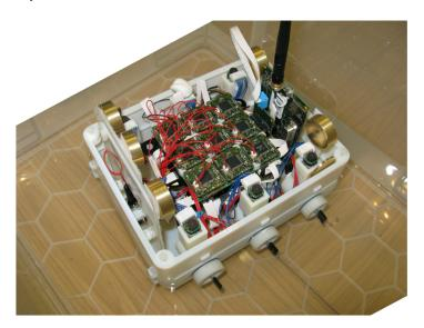
**Figure 1.** Physical platform. The physical cellular automata (CA) architecture is connected to six independent paddlers provided with Encoder and index hall effect sensor. It is powered by a three-cell lithium battery.
