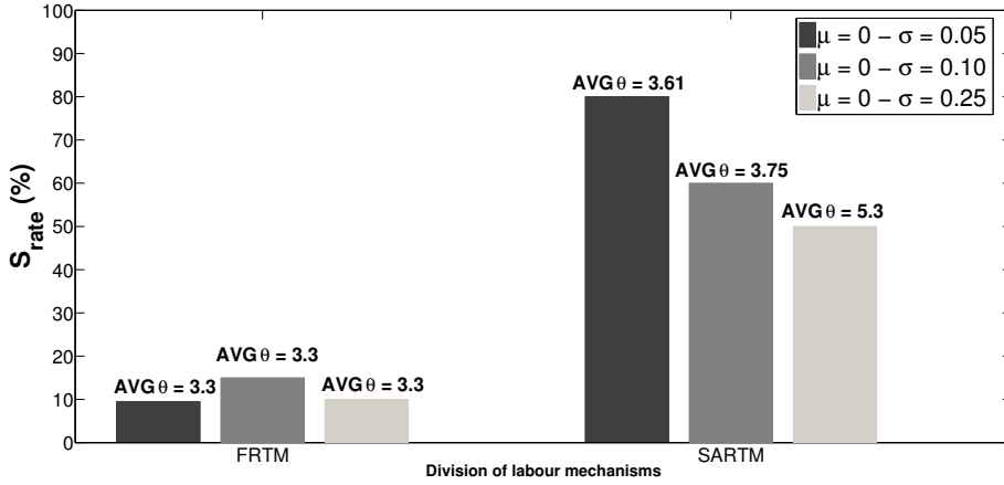
Fig. 25 ARTM and FRTM survival rates ( S_{rate} ) measured after 20 simulations runs for each experimental condition. SARTM decreases its survivability as the food sensor noise is increased. The addition of noise distributions with higher \sigma produce an increment in the average \theta threshold.
