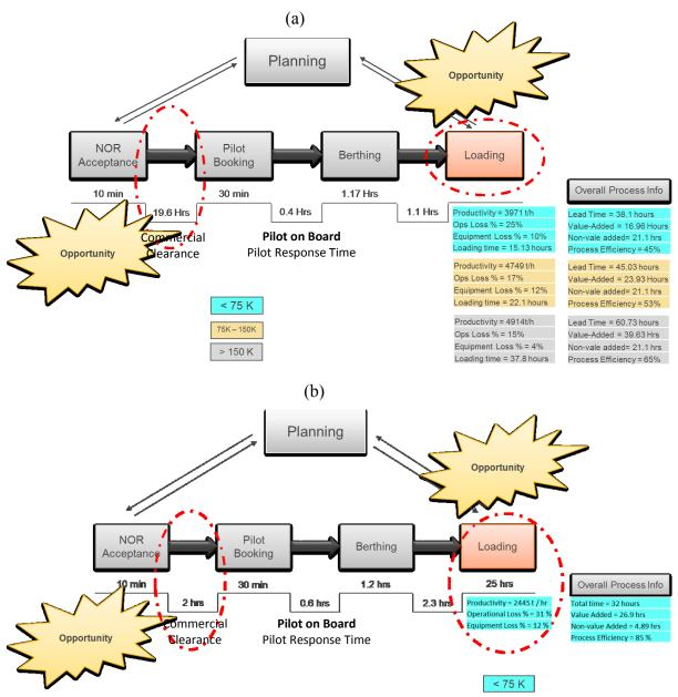
Figure 20. Analysis of Value Stream Maps for (a) iron ore pellets and (b) sinter feed
