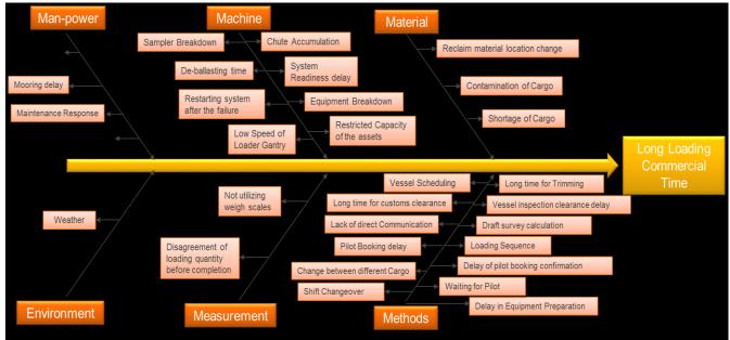
Figure 9. Cause-and-effect analysis for long ship loading commercial time
