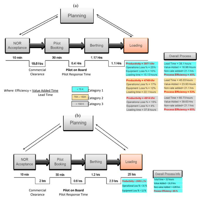
Figure 8. Value Stream Maps for (a) iron ore pellets and (b) sinter feed
