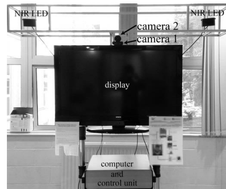
Fig. 8. System structure for the 2D+3D imaging system
