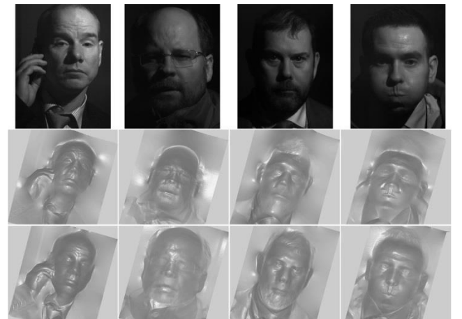
Fig. 4. 3D face reconstructions for 4 subjects from the Photoface database using the two-source PS and the standard 4-source PS methods. Top to bottom: one of the PS images, reconstructions by the two-source PS and reconstructions by the standard PS.
