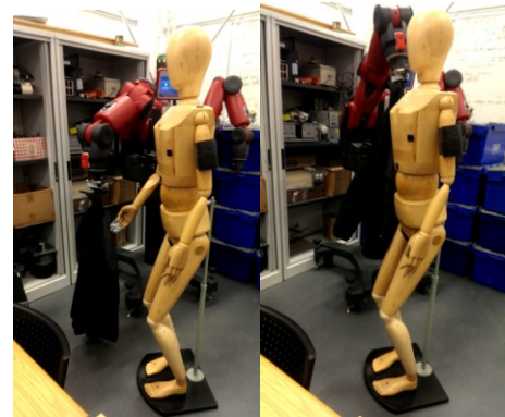
Figure 3. Sensor being tested during a dressing task. The sensor can be seen attached to the right arm near the end effector.
