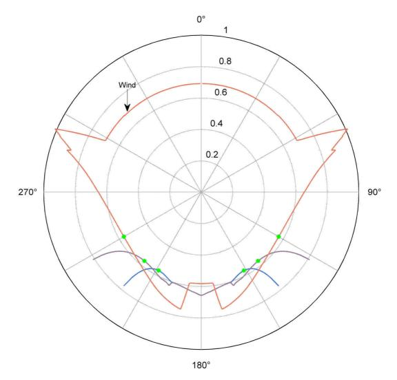
Figure VII.13: Evolution of the required friction velocity  $u_*$  (radius in m/s), with the net travelling direction  $\psi_{net}$ , for different surface roughness  $z_0$ . In blue,  $z_0=0.4$  mm, in purple  $z_0=1$  cm (baseline case) and in red,  $z_0=25$  cm. Green dots correspond to simulation cases of unconstrained in  $\psi_{net}$ , which yield, for each value of  $z_0$ , the lowest  $u_*$ .
