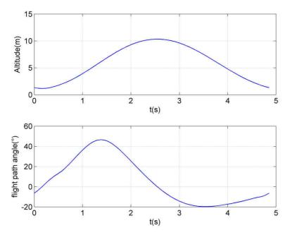
Figure VII.18: Evolution of the altitude and  $\gamma_i$  with time, for *Mariner*, along the flight path that minimizes  $Co_s$ .
