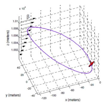
Figure II.3: Dynamic Soaring closed-loop within a linear gradient, reproduced with permission from Grenestedt *et al.* [57], © 2011 IEEE.
