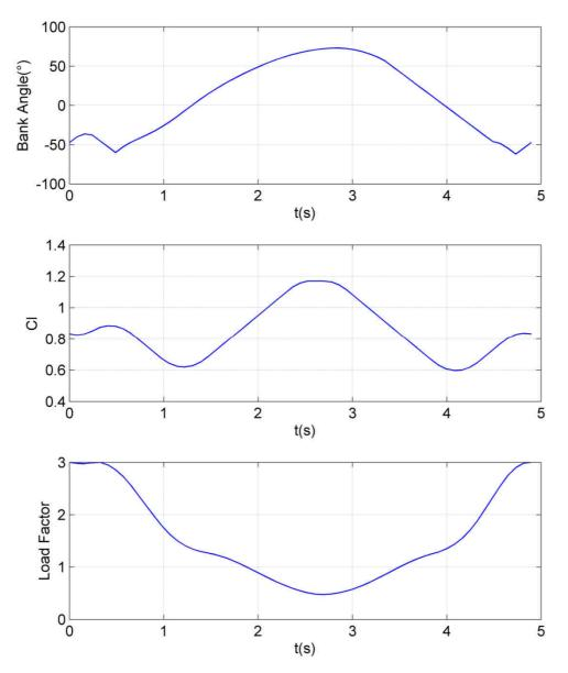
Figure VII.5: Evolution of the bank angle, the lift coefficient and the load factor with respect to time, for *Mariner*, for the case pictured in Fig. VII.4.
