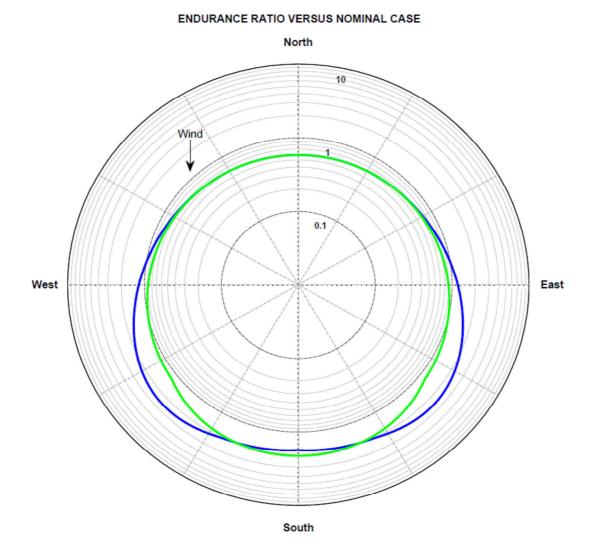
Figure VII.23: Variation of the range ratio with respect to the net heading angle, compared to the straight line case, for  $u_*=54.7$  cm/s, which corresponds to a wind strength of 8 m/s at an height of 10 metres. In green, results from straight line, in blue, results from DS.
