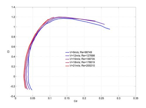
Figure III.8: Evolution of the coefficient of lift versus the coefficient of drag for the *DT-18*, for different wind tunnel speeds and their associated Reynolds number for the vehicle.
