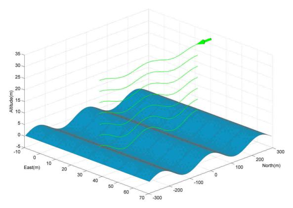
Figure III.12: Streamlines, pictured in a 2D plane, viewed from a reference frame translating at wave celerity. The wind direction is pictured by the green arrow.
