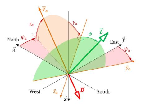
Figure IV.4: Orientation of the airspeed and of aerodynamic forces, with respect to the reference frame  $\Re_{0}.$
