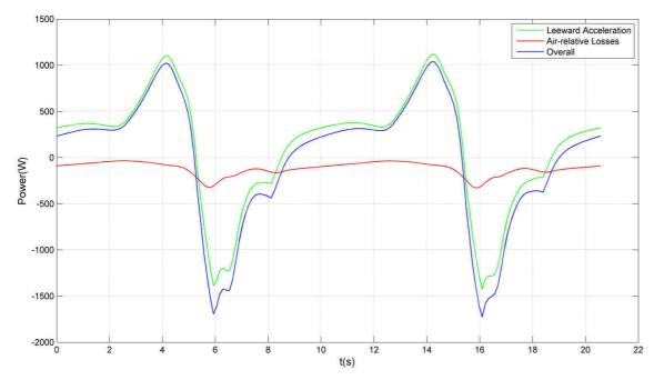
Figure V.8: Variation of power input contributions, with respect to time.
