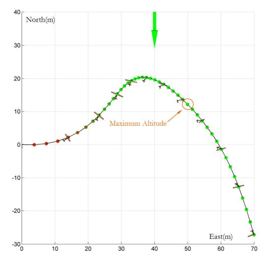
Figure V.17: Top and zoomed-in view of the open loop displayed in Fig. V.13, where the specific point of maximum altitude is encircled in orange.
