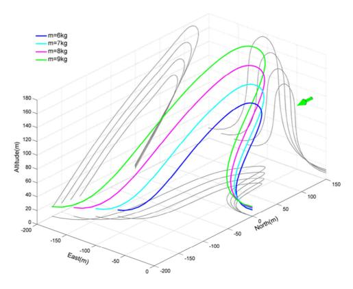
Figure VI.2: Optimal open-loop trajectories, minimizing the required wind gradient  $\beta$ , obtained for four vehicle mass, at the same wing area. For all cases,  $\bar{\rho} = 35.93 + /-0.02$ .
