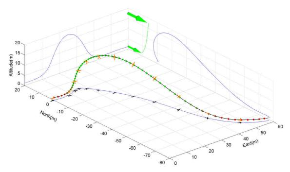
Figure VII.1: Energy-neutral open loop obtained for the *DT-18*. It takes 6.90 seconds to complete the cycle that is achieved for a minimum required friction velocity of 76  $cms^{-1}$ , which corresponds to a wind strength of 12.80  $ms^{-1}$  at a height of 10 metres. The vehicle is pictured at a 1.5:1 scale.
