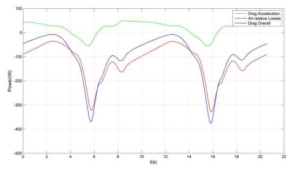
Figure V.9: Variation in power input contributions from the drag, with respect to time.
