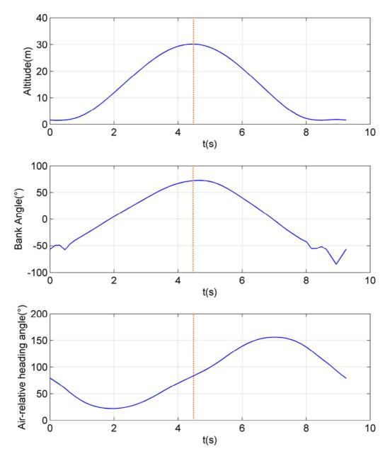
Figure V.16: Evolution of  $-z \phi$  and  $\psi_{air}$  during the cycle plotted in Fig. V.13. The point of maximum altitude is highlighted in dashed orange lines.
