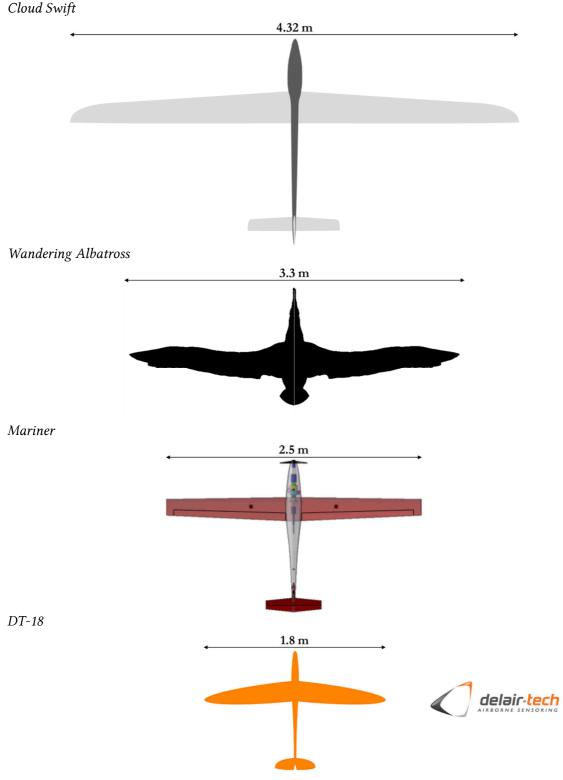
Figure III.1: Planforms of the UAVs considered, on the same scale. From top to bottom, *Cloud Swift* [19], *Wandering Albatross, Mariner*, reproduced from Bower [67], *DT-18*, reproduced from Delair-Tech [69].
