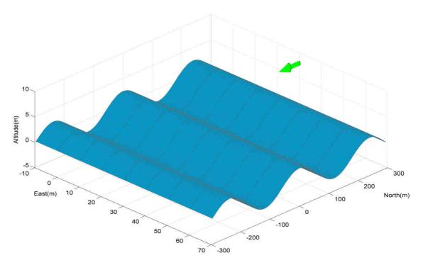
Figure III.11: Aspect of a sinusoidal wave induced by a wind blowing from the North. The wind direction is pictured by the green arrow
