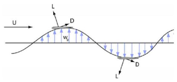
Figure II.4: Fundamental concepts of gust soaring, with the vehicle performing pull-ups within an updraft and pulling negative acceleration during downdrafts. Adapted from Patel *et al.* [62].
