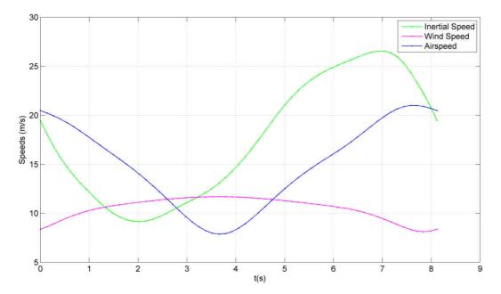
Figure VII.9: Evolution of the inertial speed, the airspeed and the local wind speed encountered by *Cloud Swift* along its optimized path, for the case pictured in Fig. VII.7.
