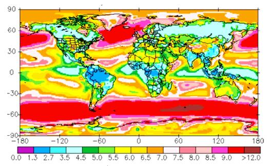
Figure I.8: Estimate of wind velocity (m.s<sup>-1</sup>) at 50m, average over a 10-year period [37]. These data were obtained from the NASA Langley Research Center Atmospheric Science Data Center Surface meteorological and Solar Energy (SSE) web portal supported by the NASA LaRC POWER Project.
