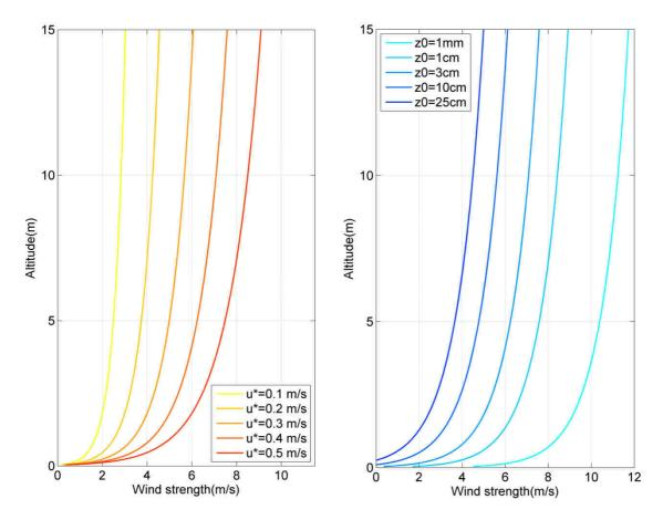
Figure III.10: Influence of variables from Eq. III.17 on the main wind profile. Left, variations in friction velocity for values representative of the atmospheric boundary layer. Right, variations in surface roughness length, representative, from the lowest to the highest, of open sea, open tarmac, open grass, low crops, and high crops respectively.
