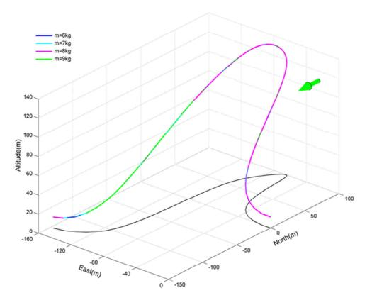
Figure VI.1: Optimal open-loop trajectories, minimizing the required wind gradient  $\beta$ , obtained for four vehicle mass, at the same wing loading. For all cases, the wing loading is 141.6 N/m<sup>2</sup>, the wind gradient is  $\beta = 0.1076 \text{ s}^{-1}$  and  $\bar{\rho} = 35.93$ .
