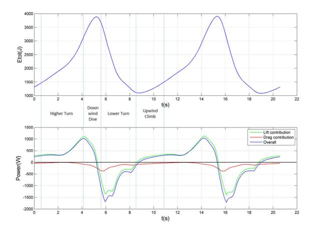
Figure V.6: Variation in total energy with time and in the associated rate of energy with time
