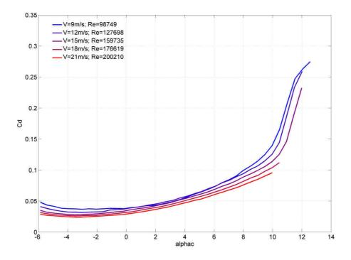
Figure III.7: Evolution of the coefficient of drag with the angle of attack (*alphac*) for the *DT-18*, for different wind tunnel speeds and their associated Reynolds number for the vehicle.
