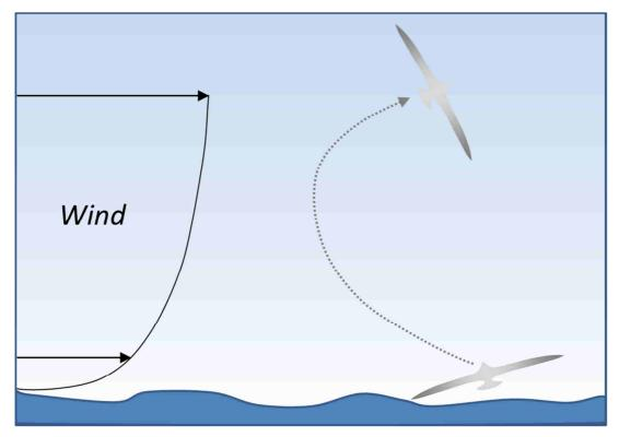
Figure I.17: Schematic 2D display of a dynamic soaring path within the wind shear gradient.
