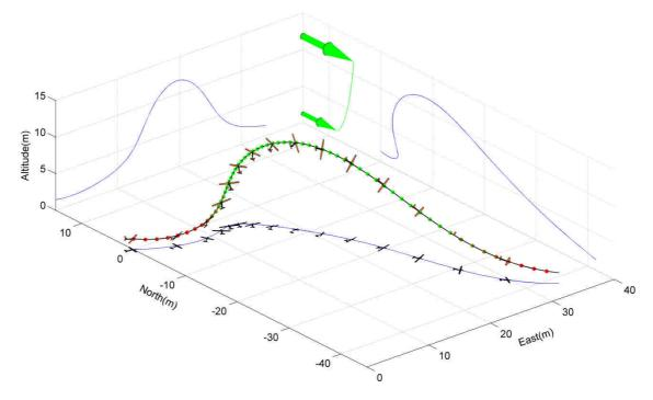
Figure VII.4: Energy-neutral open loop obtained for the *Mariner*. It takes 4.90 seconds to complete the cycle that is achieved for a minimum required friction velocity of 56.7 cm.s<sup>-1</sup>, which corresponds to a wind strength of 9.55 m.s<sup>-1</sup> at a height of 10 metres. The vehicle is pictured at a 1:1 scale.
