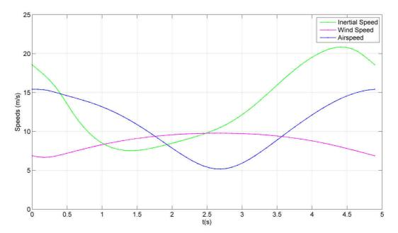
Figure VII.6: Evolution of the inertial speed, the airspeed and the local wind speed encountered by *Mariner* along its optimized path, pictured in Fig. VII.4.
