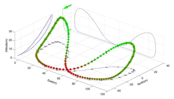
Figure V.7: Overall energy-harvesting strategy. The energy neutral closed loop trajectory from Fig. IV.1 is coloured following a red to green scale as a function of the local power input. Total energy is extracted at green-coloured positions and is lost at red-coloured positions.
