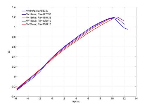
Figure III.6: Evolution of the coefficient of lift with the angle of attack (alphac) for the *DT-18*, for different wind tunnel speeds and their associated Reynolds number for the vehicle.
