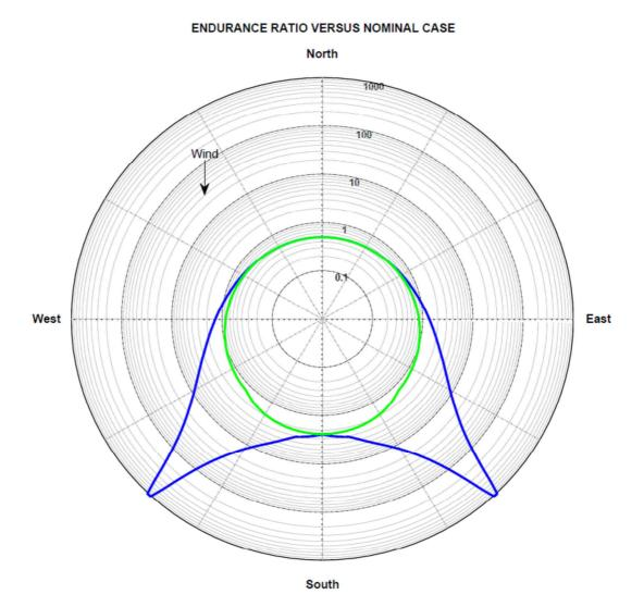
Figure VII.21: Variation of the range ratio with respect to the net heading angle, compared to the straight line case, for  $u_*=66$  cm/s, which corresponds to a wind strength of 10 m/s at an height of 10 metres. In green, results from straight line, in blue, results from DS.
