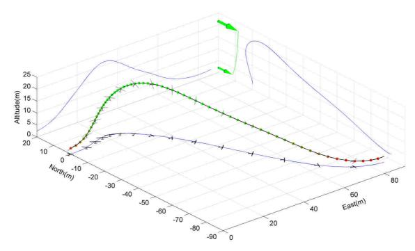
Figure VII.7: Energy-neutral open loop obtained for *Cloud Swift*. It takes 8.12 seconds to complete the cycle that is achieved for a minimum required friction velocity of  $62.4 \text{ cm.s}^{-1}$ , which corresponds to a wind strength of  $10.52 \text{ m.s}^{-1}$  at a height of 10 metres. The vehicle is pictured at a 1:1 scale.
