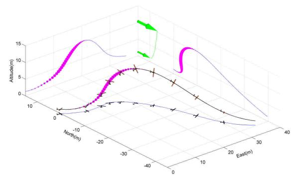
Figure VII.16: Thrust-augmented-energy-neutral open loop obtained for *Mariner*, achieved within 4.86 seconds, for  $u_* = 47.5 \text{ cm.s}^{-1}$ . The pink-coloured dots are proportional, in size, to the intensity of the thrust provided by the vehicle. The vehicle is pictured at a 1:1 scale.
