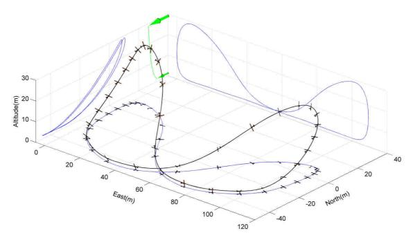
Figure V.1: Closed loop energy neutral trajectory obtained for a wing tip clearance of 50 cm, a surface roughness length of 3 cm and a wind friction velocity of 80 cm/s, which corresponds to a wind speed of 11.34 m/s at 10 metres. The trajectory is completed in 20.58 seconds. The wind profile and direction is represented by the green arrow. The scale of the vehicle (Mariner) is augmented by a factor 1.5 for better visibility.
