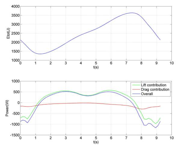
Figure V.15: Variation in total energy along the path, with the associated evolution of power contributions over time.
