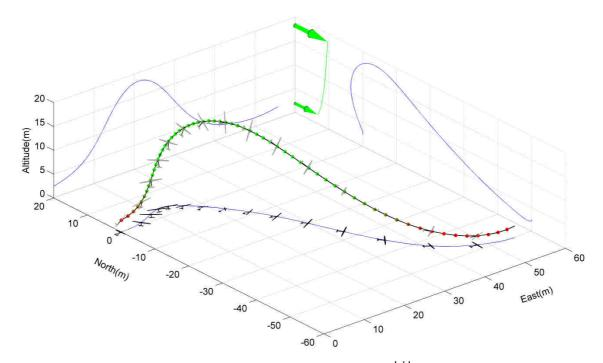
Figure VII.10: Energy-neutral open loop obtained for *Cloud Swift* for  $|\dot{\phi}| \leq 60^{\circ}/s$ . It takes 6.01 seconds to complete the cycle that is achieved for a minimum required friction velocity of 52.2 cm.s<sup>-1</sup>, which corresponds to a wind strength of 8.80 m.s<sup>-1</sup> at a height of 10 metres. The vehicle is pictured at a 1:1 scale.
