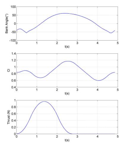
Figure VII.17: Evolution of  $\phi$ ,  $C_L$  and T with time, for *Mariner*, along the flight path that minimizes  $Co_s$ .
