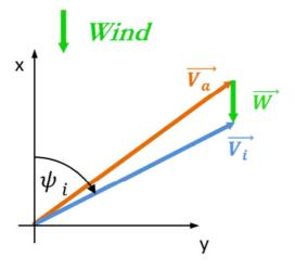
Figure VII.19: Top schematic view of the triangle of speed, between inertial speed, wind speed and airspeed, for a given inertial speed heading and a given wind speed.
