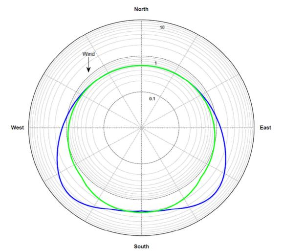
Figure VII.22: Variation of the range ratio with respect to the net heading angle, compared to the straight line case, for  $u_*=59.4$  cm/s, which corresponds to a wind strength of 9 m/s at an height of 10 metres. In green, results from straight line, in blue, results from DS.
