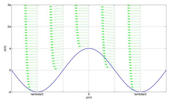
Figure III.13: Velocity profiles of the wind component due to the wave curvature. The vertical amplitude scale of the wave is voluntarily exaggerated.
