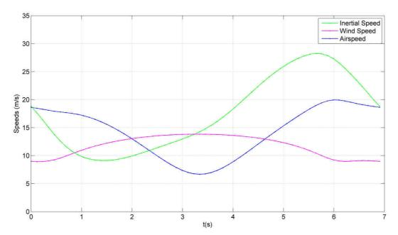
Figure VII.3: Evolution of the inertial speed, the airspeed and the local wind speed encountered by the *DT-18* along its optimized path, pictured in Fig. VII.1.
