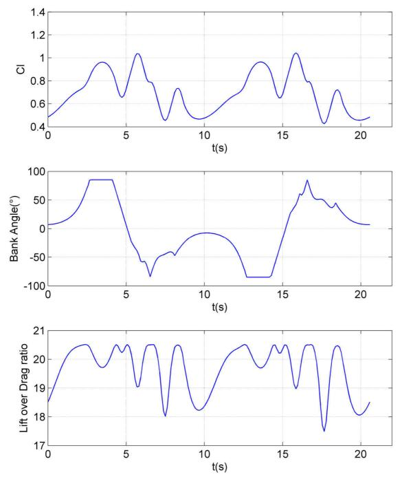
Figure V.4: Evolution of  $C_L$ ,  $\phi$  and  $C_L/C_D$  over time.
