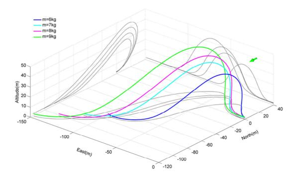
Figure VI.7: Three dimensional trajectories optimized to minimize the wind strength required, for different vehicle mass.  $\bar{\rho} = 0.0113$  for all cases.
