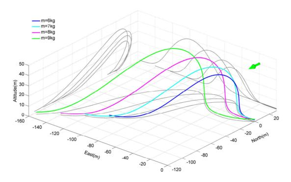
Figure VI.9: Three dimensional trajectories optimized to minimize  $\overline{Co_s}$ , for different vehicle mass.  $\overline{Co_s} = 0.015$  and  $\overline{\rho} = 0.00952$  for all cases.
