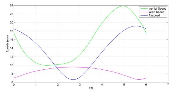
Figure VII.12: Evolution of the inertial speed, the airspeed and the local wind speed encountered by *Cloud Swift* along its optimized path, for a maximum rolling rate of 60°/s, corresponding to Fig. VII.10.
