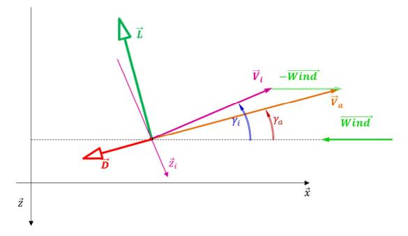
Figure V.5: Orientation of speeds and forces for a 2D-simplified windward climb. The lift is tilted by an angle  $(\gamma_i - \gamma_a)$  towards the direction of motion  $\vec{x}_i$ . This entails a positive working component which governs the energy extraction.
