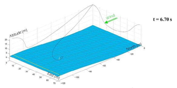
Figure V.18: Evolution of the vehicle above a wave.  $u_* = 0.57$  m/s; a = 2.47 m;  $\lambda = 193$  m; c = 17.5 m/s.
