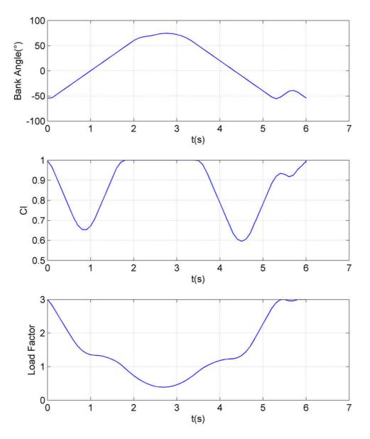
Figure VII.11: Evolution of the bank angle, the lift coefficient and the load factor with respect to time, for *Cloud Swift*, with a maximum rolling rate of  $60^{\circ}$ /s, corresponding to the flight path pictured in Fig. VII.10.
