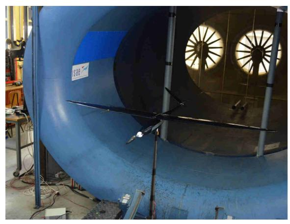
Figure III.5: The *DT-18* experimental mock-up into place, through the single ventral mast, inside the elliptical test section of the *S4* wind tunnel. The open test section is clearly visible, as the workshop is visible (left) outside of the section. The suction fans are visible (top right) at the end of the suction chamber, leeward of the diffuser. The curved rails of the cradle can also be seen (bottom), as well as the external feed (bottom left) for powering on board electronics.
