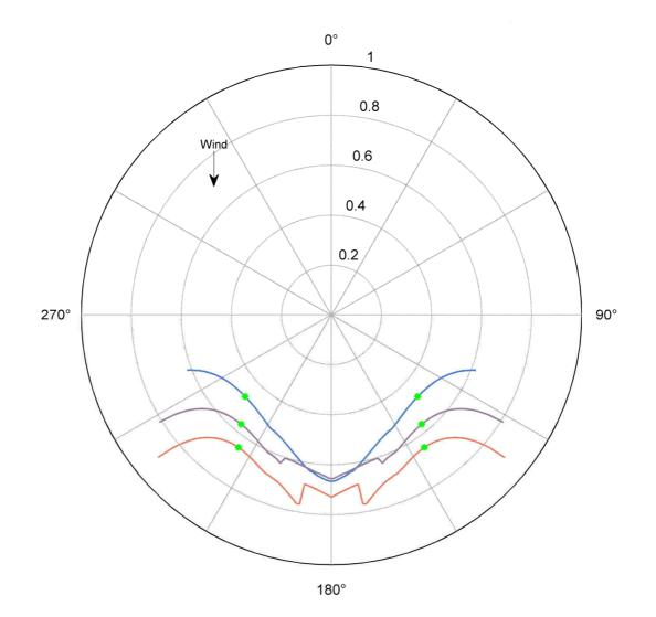
Figure VII.15: Evolution of the required friction velocity  $u_*$  with the net travelling direction  $\psi_{net}$ , for different ground clearance  $G_{clear}$ . In blue,  $G_{clear}=0$  cm, in purple  $G_{clear}=50$  cm (baseline case) and in red,  $G_{clear}=1$  m. Green dots corresponds to the simulation case unconstrained in  $\psi_{net}$ , which yield, for each value of  $G_{clear}$ , the lowest  $u_*$ .
