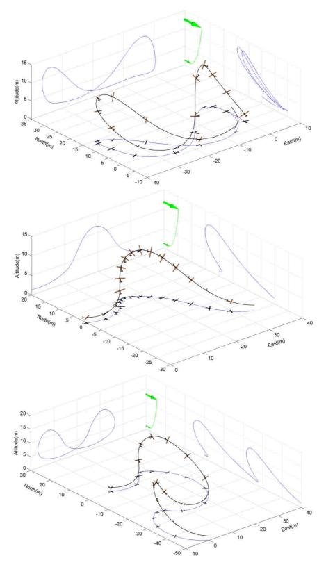
Figure VII.14: Solution cases corresponding to Fig. VII.13, for  $z_0=25 \text{ cm}$ . Top: net flight path heading 0°, directed windward,  $u_*=69.2 \text{ cm/s}$ ,  $V_{net}=0.4 \text{ m/s}$ . Middle: net flight path heading 120°, minimal  $u_*=56.7 \text{ cm/s}$ ,  $V_{net}=8.0 \text{ m/s}$ . Bottom: net flight path heading 180°, directed leeward,  $u_*=58.2 \text{ cm/s}$ ,  $V_{net}=4.8 \text{ m/s}$ .
