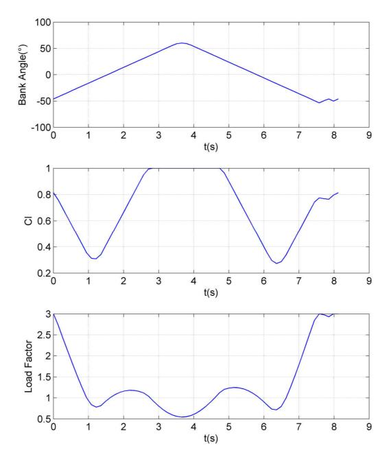
Figure VII.8: Evolution of the bank angle, the lift coefficient and the load factor with respect to time, for *Cloud Swift*, for the case pictured in Fig. VII.7.
