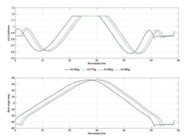
Figure VI.6: Evolution of control variables over dimensionless time, obtained by minimizing the required friction velocity, for various mass at a fixed wing loading of 141.6  $N/m^2$ .  $\bar{\rho} = 0.0113$  for all cases.
