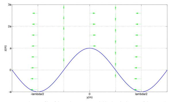
Figure III.14: Velocity profiles of the wind component entailed by the orbital motion of the wave. The velocity scale is five time that of Fig III.13.
