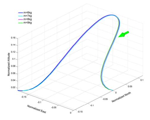
Figure VI.3: Three dimensional curves, plotted in dimensionless coordinates, obtained by minimizing the required wind gradient  $\beta$ , for four vehicle mass, at the same wing area. For all cases,  $\bar{\rho} = 35.93 \pm -0.02$
