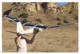
Figure I.3: *Qinetiq Zephyr*, a solar-powered, 18 metres-wingspan-UAV, which sustained flight for two weeks in July 2010.
