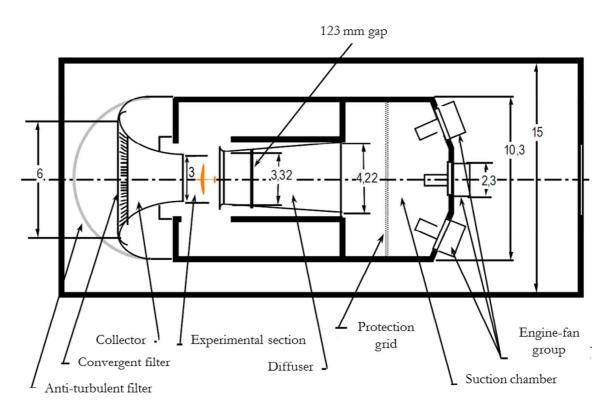
Figure III.2: Top view of the *S4* wind tunnel. All distances are in *m*, unless otherwise stated. The DT-18, colored in orange, is schematically included in the test section. Adapted from [74].
