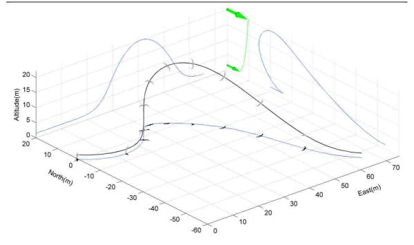
Figure IV.5: Energy-neutral trajectory for conditions representing Sachs [47]. The surface is rather flat with  $z_0=3$  cm. The wind friction velocity required to sustain DS is 60.6 cm/s, the duration is 7 seconds.
