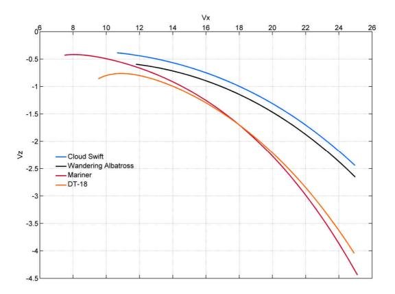
Figure III.9: Comparison of speed polar for each of the four vehicles.
