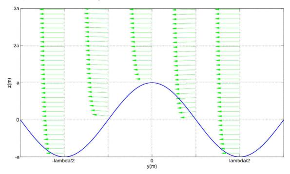
Figure III.15: Velocity profiles of the wind established over a moving wavy surface.
