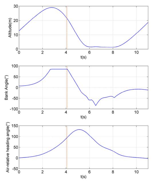
Figure V.12: Evolution of -z,  $\phi$  and  $\psi_{air}$  during the first half of the cycle plotted in Fig. V.1. The moment of maximum power input is highlighted in dashed orange lines.
