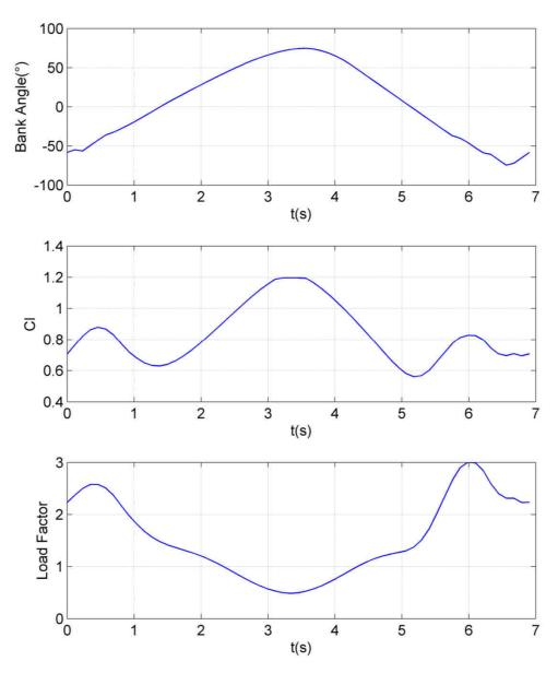
Figure VII.2: Evolution of the bank angle, the lift coefficient and the load factor with respect to time, for the *DT-18*, for the case pictured in Fig. VII.1.
