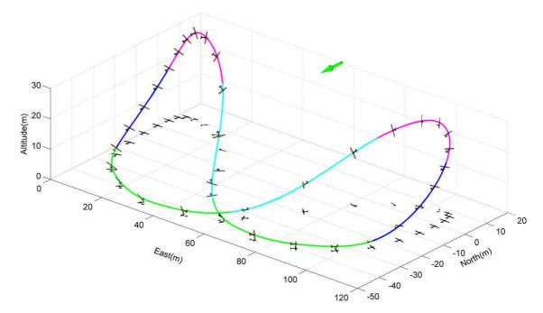
Figure V.2: Phases of flight are evidenced out using different colours. Blue for the upwind climb, magenta for the high turn, cyan for the downwind dive and green for the lower turn.
