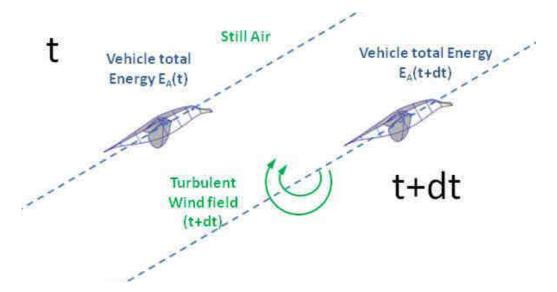
Figure IV.2: Energy transfer from a wind based point of view.
