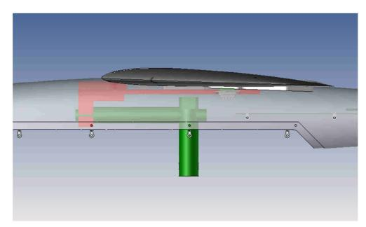
Figure III.3: Rendering of the mechanical set-up of the mock-up on the mast. The holding plate (red), supports the mock-up on its upper surface and clasp the measurement-unit (horizontal, green) in one of its forward extremity. The measurement-unit is encircled at its aft extremity by the ventral mast (vertical, green). Copyrights *Delair-Tech*.
