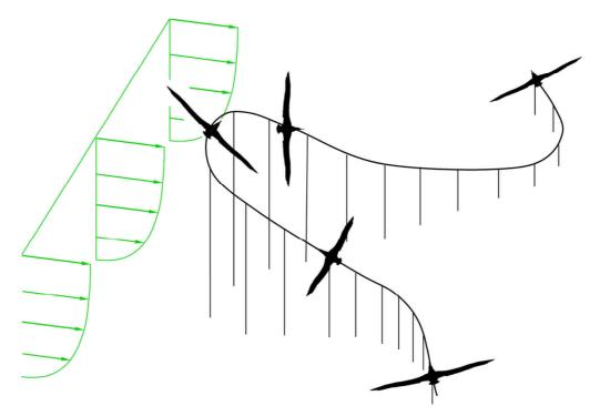
Figure I.18: Overall aspect of a dynamic soaring trajectory.
