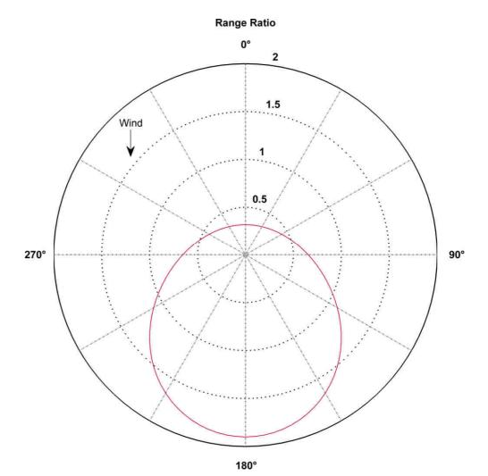
Figure VII.20: Evolution of the range ratio versus the flight heading, for a given wind. Chart obtained for *Mariner*, flying in straight line, under a wind strength of 8  $m.s^{-1}$ .
