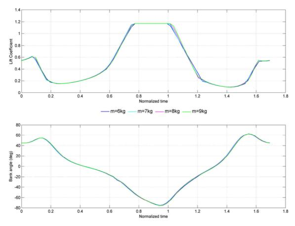
Figure VI.4: Evolution of control variables over dimensionless time, obtained by minimizing the required wind gradient  $\beta$ , for four vehicle mass, at the same wing area. For all cases,  $\bar{\rho} = 35.93 + -0.02$ .
