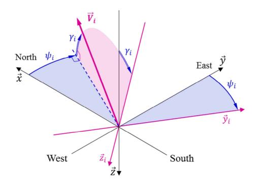
Figure IV.3: Orientation of the inertial speed with respect to the reference frame  $\Re_0$
