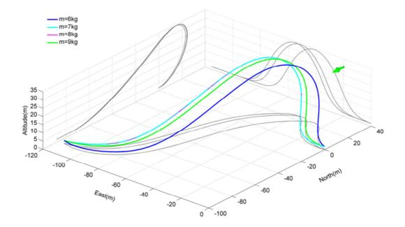
Figure VI.5: Optimal open-loop trajectories, minimizing the required friction velocity for various mass at a fixed wing loading of 141.6  $N/m^2$ .  $\bar{\rho} = 0.0113$  for all cases,  $z_0$  was unchanged at 3 cm.
