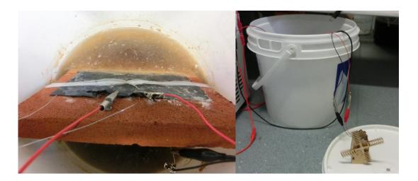
*Figure 9.10* MFC made out of terracotta floor tile placed in the bucket filled with wastewater (left) and the same MFC directly energizing the windmill motor (right).
