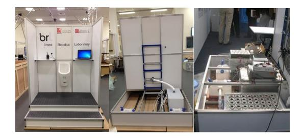
Figure 5.42 Urinal design in Reinvent the Toilet Fair in India (left, middle) with 40 ceramic MFCs placed inside the tank (right).
