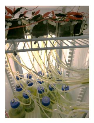
Figure 4.5 MFCs and bioreactors in temperature controlled light incubator.
