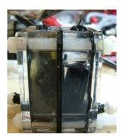
Figure 2.5 Single-chamber MFC with open to air cathode (left) and two-chamber MFC with aqueous cathode (right).
