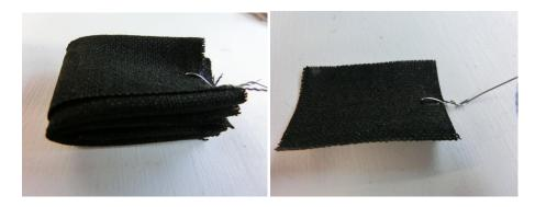
Figure 2.2. MPL (Microporous layer) on carbon cloth used as folded and single layer electrode
