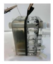
Figure 5.1 Experimental set up. Left: control MFC with carbon veil electrode in the cathode half-cell, right: single layer MPL coated carbon cloth pressed against the membrane.
