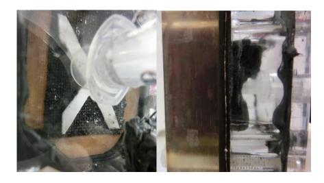
Figure 5.16 Catholyte formation in situ on the electrode surface as droplets on 2D electrode (left) and in 3D electrode sponge (right). Formed droplets are more visible on 2D structure.
