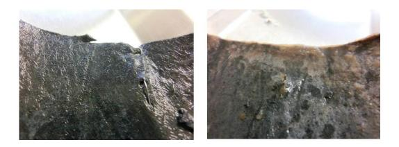
Figure 5.40 Cathode electrode on the air side. No visible biofilm growth was observed in working MFC (left) compared to visible biofilm formed in MFC left in open circuit (right).
