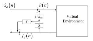
Fig. 7: Control architecture of the ISS approach for impedance-type haptic displays [1]
