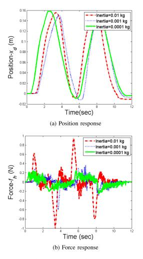
Fig. 13: Experimental results with the proposed ISS approach; (a) Position responses (m = 0.0001 kg), (b) Force responses.
