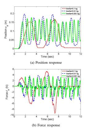
Fig. 3: Low inertia rendering experimental results; (a) Position response, (b) Force response.
