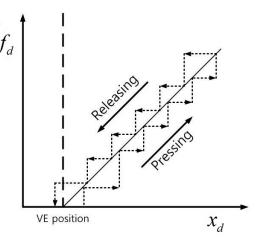
Fig. 5: Position vs. force trajectory of an impedance-type haptic interface in single contact and separation motion. Signals are captured in between haptic device and discrete interface.
