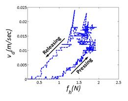
Fig. 10: Input (measure human force,  $f_h$ ) vs. output (desired velocity,  $V_d$ ) behavior of the partial admittance model.
