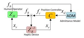
Fig. 8: Block diagram representation of an admittance-type haptic interface.
