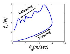
Fig. 11: Input (The velocity tracking error,  $\dot{e}_d$ ) vs. output (the controller force,  $f_c$ ) behavior of the integrator and position controller.
