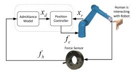
Fig. 1: Conceptual representation of an admittance-type haptic interface
