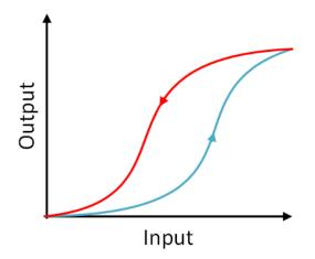
Fig. 6: A graphical illustration of input-output behavior from a counterclockwise hysteresis.
