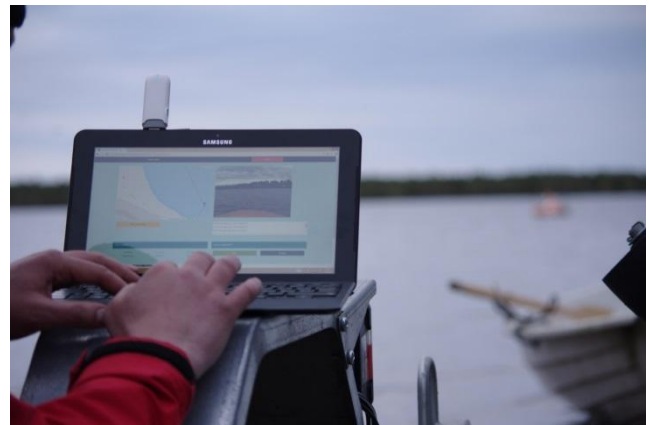
Figure 10. Ground control station with the web-interface to the USV.
