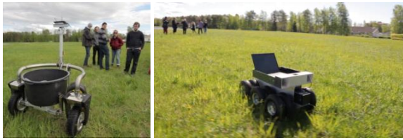
Figure 4. The land robots in the outside testing area; The C-frame robot platform on the left and the Mörrri robot on the right.
