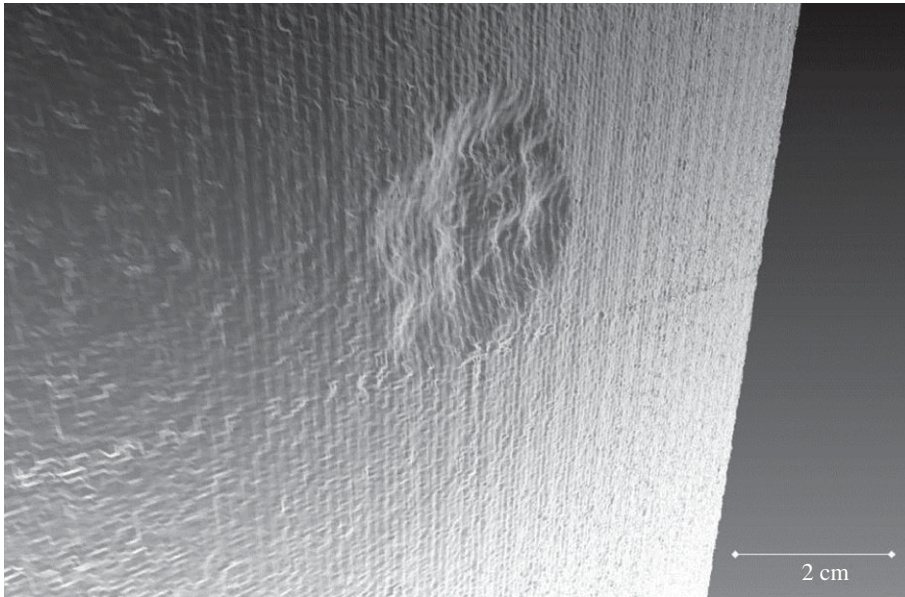
Figure 5. Mephisto Eos 3D scan of a bullet impact on the stone surface (not treated with Wacker OH 100).
