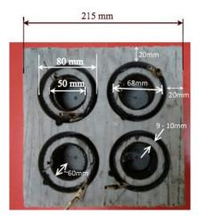
Figure 1: Aerobic setup. View of the concrete block with four bio-reactors.
