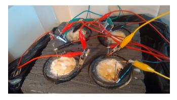
Figure 2: Photo of one block with four aerobic bio-reactors each, in the process of recording electrical potential of the cells.
