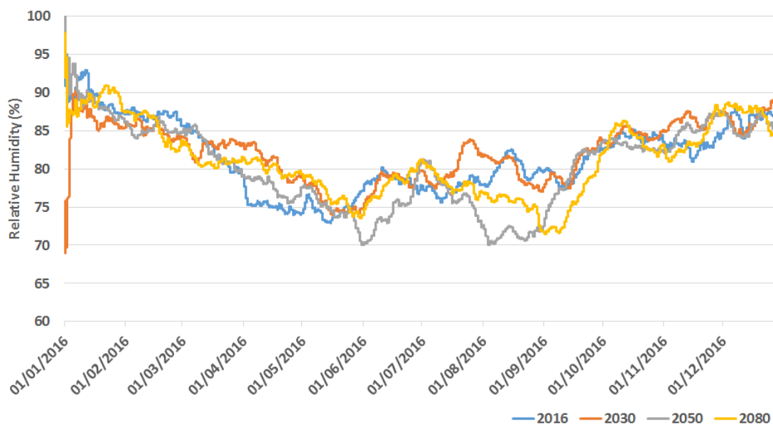
Figure 13 Simulated annual relative humidity for Bristol in 2016, 2030, 2050 and 2080, displayed with a monthly moving average.
