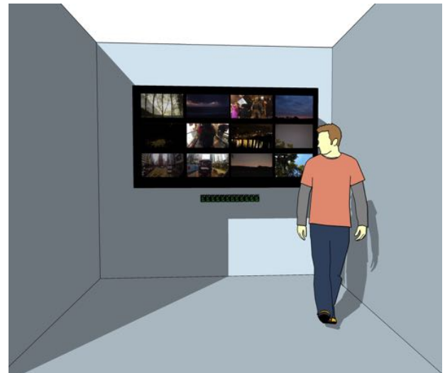
Figure 1: Standard 'flat' installation using matrix of 12 monitors showing Raspberry Pi driving computers.
