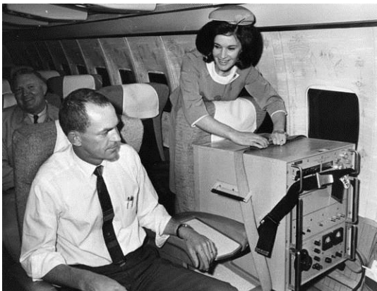
Figure 1: A caesium beam timepiece used in the US space program occupies a first-class seat aboard a TWA flight from London to Washington on November 23, 1966; this formed part of the famous Hafele-Keating experiment published in 1972 (Photo: Jackson, Getty Images)
