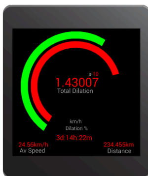
Figure 8: Early prototype design for AndroidWear form showing current dilation and velocity as arc readouts, accumulated dilation, average speed and distance travelled (since last reset)
