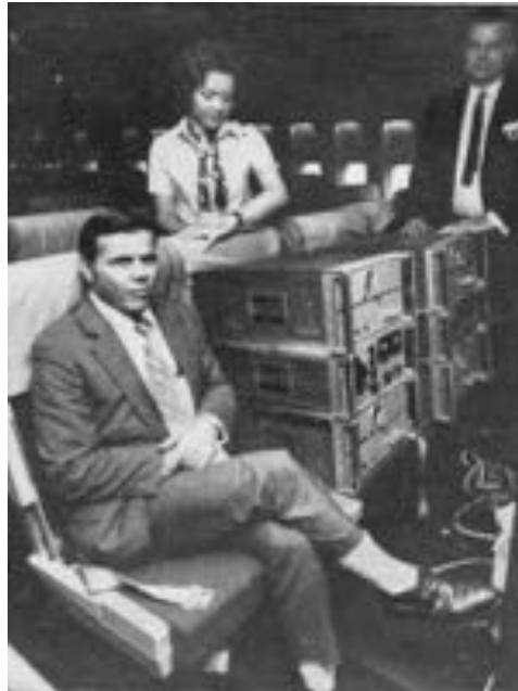
Figure 5.1: The Hafele Keating Experiment of 1971, showing a caesium beam clock aboard a commercial jet airliner. This simple but pivotal experiment gave concrete evidence to the predicted effects of time dilation.
