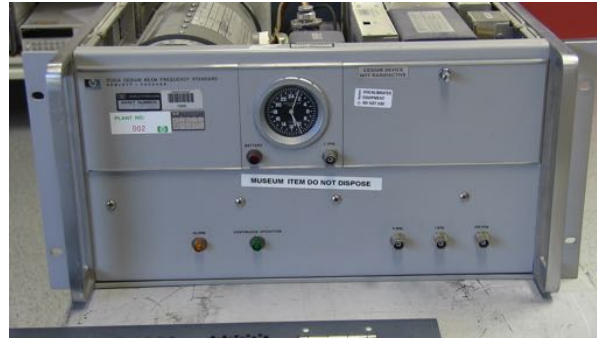
Figure 3.4: One of the actual cesium beam atomic clock units used in the 1960's 'flying clocks' experiment to synchronise time around the world. And later in the Hafele-Keating experiment to prove relativity theory. Currently kept at Agilent (formally Hewlett Packard) Melbourne headquarters.
