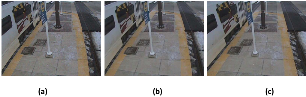
Figure 40: Example of an enhance image: (a) First of the six original frame, (b) High-Resolution Enhance image, (c) High-Resolution and undistorted Enhance image 55 .
