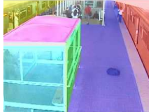
Figure 30: An example of useful segmented regions in the context of video surveillance 37 .
