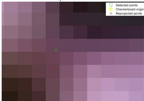
Fig. 5a. Reprojection error is the offset from the circle center to the cross intersection
