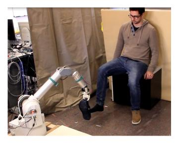
Fig. 1. Assisted-dressing scenario with a WAM robot: Use case of putting on a shoe.
