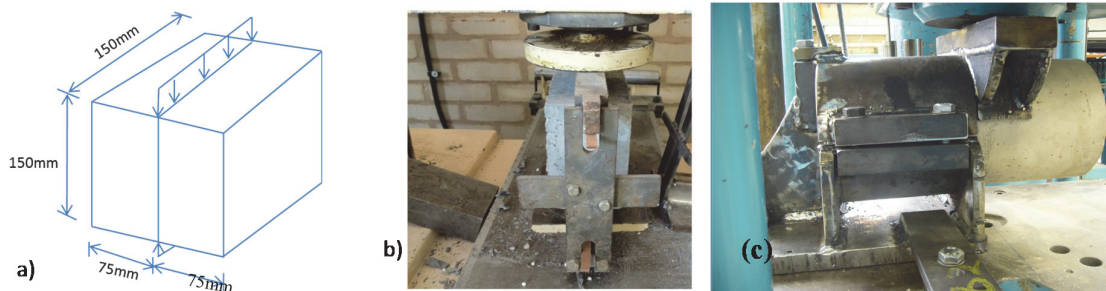
Fig. 8. a, b) Splitting (Brazilian) Tensile test and (c) Direct 100 x 100mm \phi cylinder (Guillotine) Shear test
