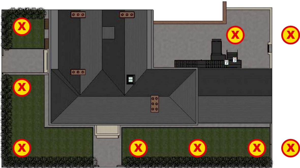
Figure 5: Scan Station locations during the laser scan of Joule House.
