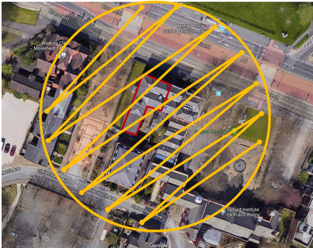
Figure 9: Path taken by drone during aerial photogrammetry of Joule House.
