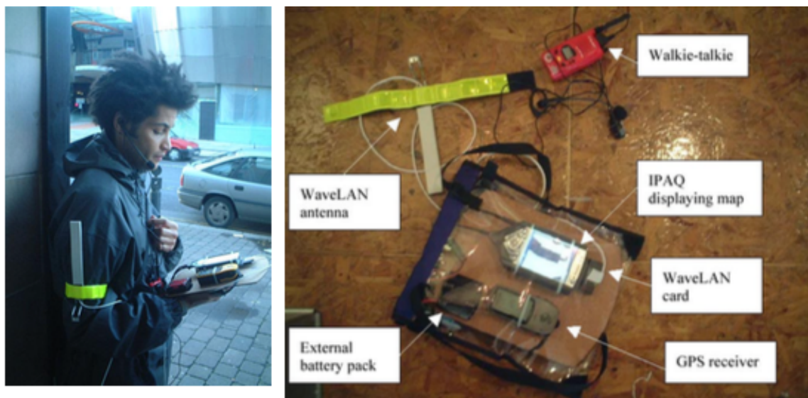
Figure 16: First iteration of Can You See Me Now? runner equipment (Anastasi et al. , 2002)
