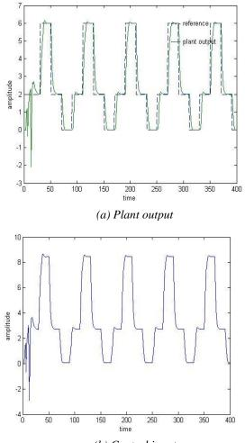
*(b) Control input Fig. 8. Plant output and control input*
