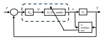
Fig. 5. Adaptive U-model control system
