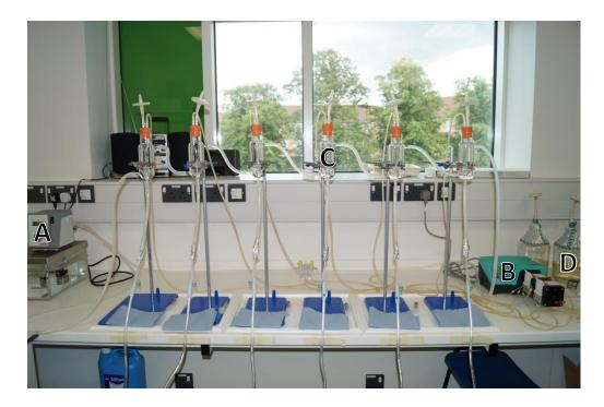
**Figure 43.** Photograph of the bladder model set up. (A) The re-circulating water bath that aimed to retain the models at 37°C, (B) the peristaltic pump that supplied the models (C) with artificial urine stored in the vented bottles (D).
