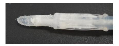
**Figure 50.** Photograph of a blocked catheter removed from the *in vitro* bladder model system. Crystalline deposits have completely occluded the eye hole and are visible on the tip and balloon. Cuffing, the creases and ridges that form as the retention balloon fails to return to its original size, is also evident.
