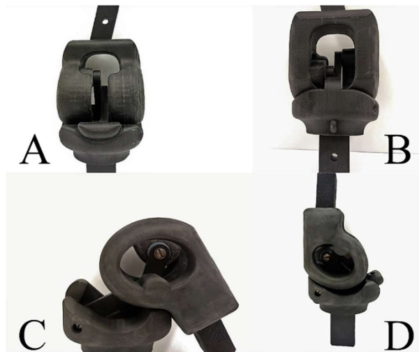
Fig. 10. Constructed joint (A) rear view, (B) front view, (C) full flexion, and (D) full extension
