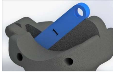
Fig. 6. Modification of the proposed tibial head preventing flexion or over extension when forces are applied superiorly
