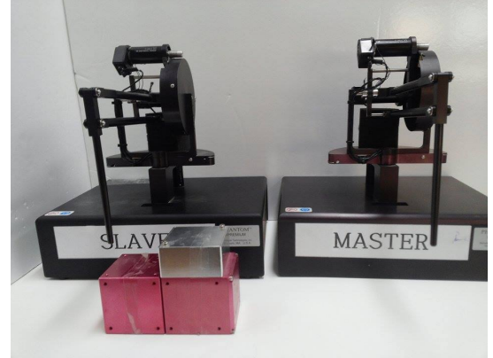
Fig. 10: The experimental teleoperation setup consisting of two Phantom Premium 1.5 robots.
