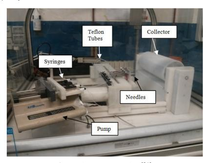
Figure 2. Electrospinning machine [21].
