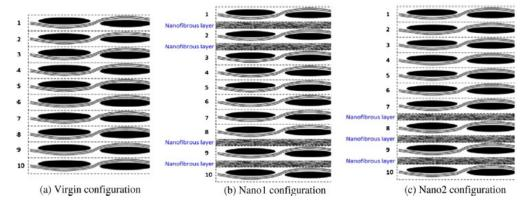
Figure 3. Two different configurations for interleaving carbon/epoxy laminates [27].
