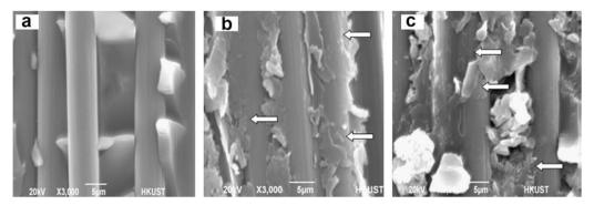
**Figure 15.** Photographs of fracture surfaces after an interlaminar shear test for CFRPs composites with different clay contents: (a) 0 wt %; (b) 3 wt % and (c) 5 wt % [132].
