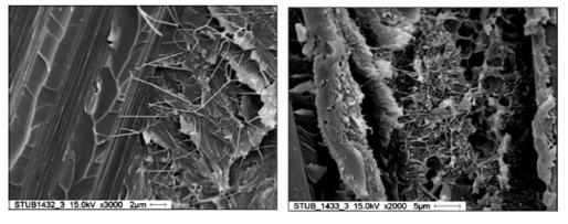
Figure 4. Toughening mechanism by NY66 [27].
