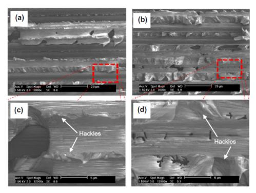
**Figure 14.** SEM of fractured Mode II DCB coupons at different magnifications for (a,c) baseline laminate and (b,d) SWCNT-modified laminate. The existence of larger hackles can be seen for SWCNT-modified laminate [73].
