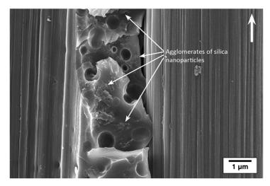
**Figure 12.** SEM image of carbon/epoxy laminate modified with silica/rubber nanoparticles (fracture surface of G<sub>IIc</sub> test specimen). The white arrow indicates the direction of crack propagation [68].
