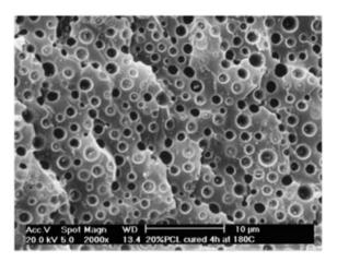
Figure 7. Phase separation in PCL/epoxy blend [49].
