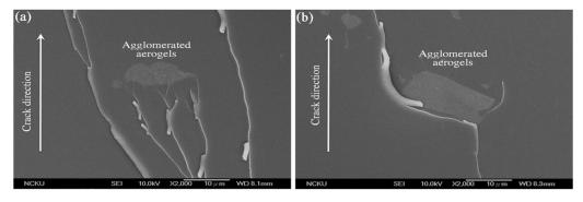
**Figure 16.** FEG-SEM images of the fracture surfaces of a composite with a carbon aerogel content of 0.5 wt %. The surfaces show (a) crack pinning and (b) crack deflection [82].
