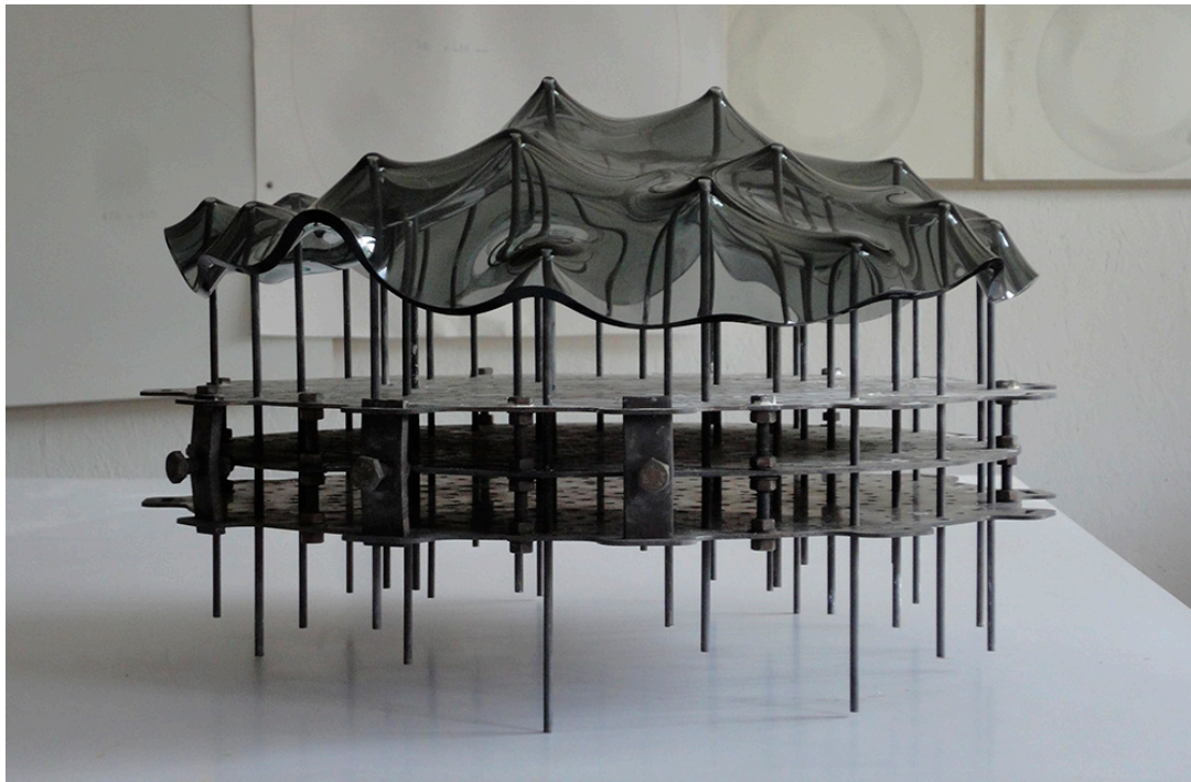
Figure 9. RPT system with a bowl formed upside down on the pins, (photo: Jorgensen, T. 2013).
