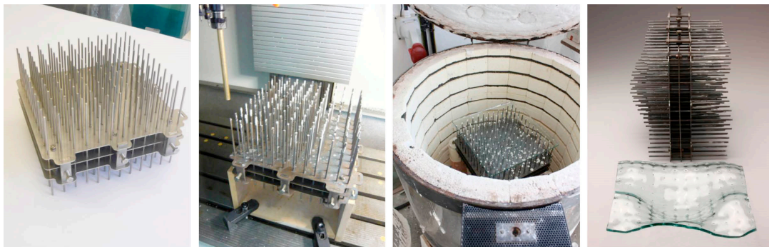
Figure 1. Initial explorations by the author of using Reconfigurable Pin Tooling (RPT) in combination with the glass-slumping technique, (photos: Jorgensen, T. 2010).
