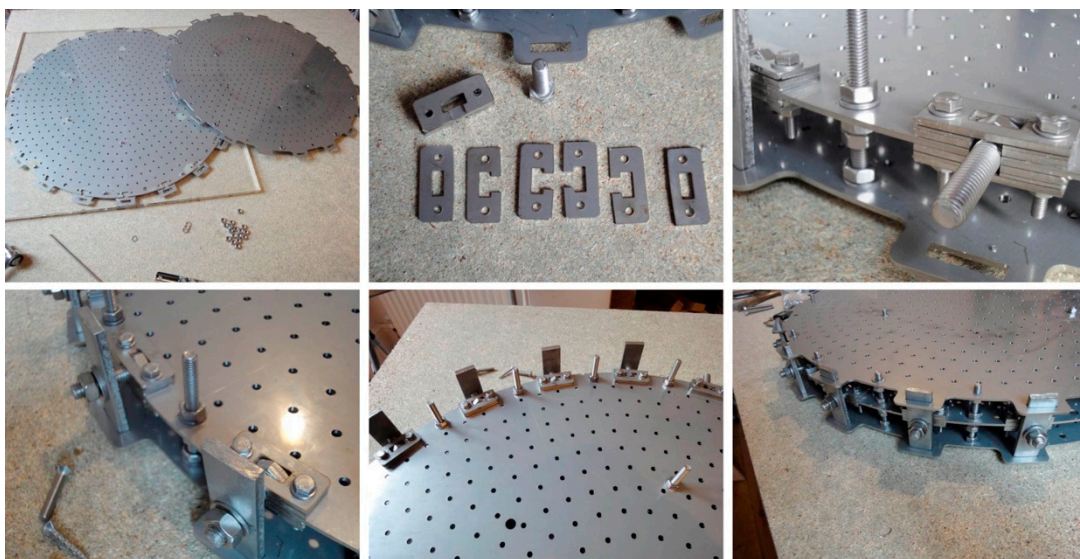
Figure 7. Construction of the improved pin locking mechanism, created using sections of laser-cut shapes layered and bolted together to create a rigid fixing point for the pressure bolts to operate from, (photos: Jorgensen, T. 2012).
