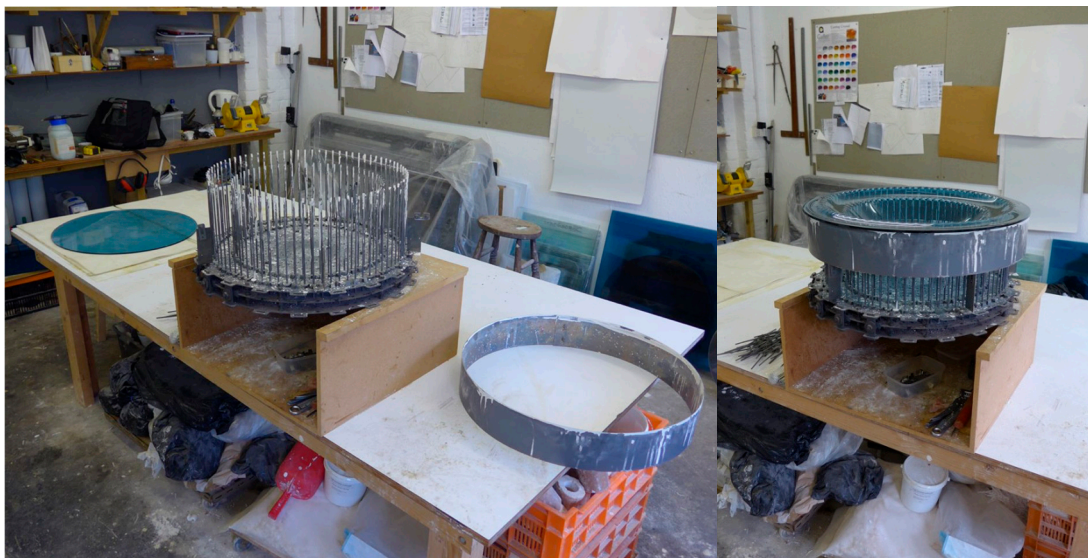
Figure 11. The second stage of the creative explorations of the glass RPT system, utilising the RPT system's underlying circular array geometry to create bowls using sets of pins positioned in concentric circles, (photo: Jorgensen, T. 2013).
